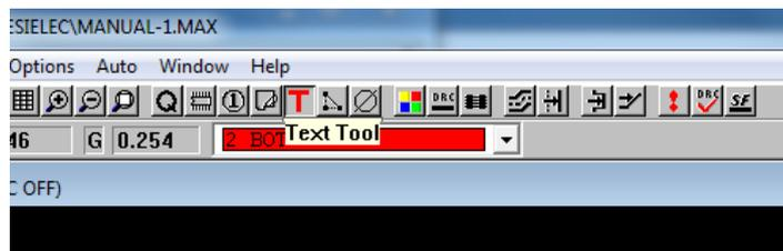
A right click will take us to the options where we can add a new piece of text. In our case the text to be inserted has a double purpose:
