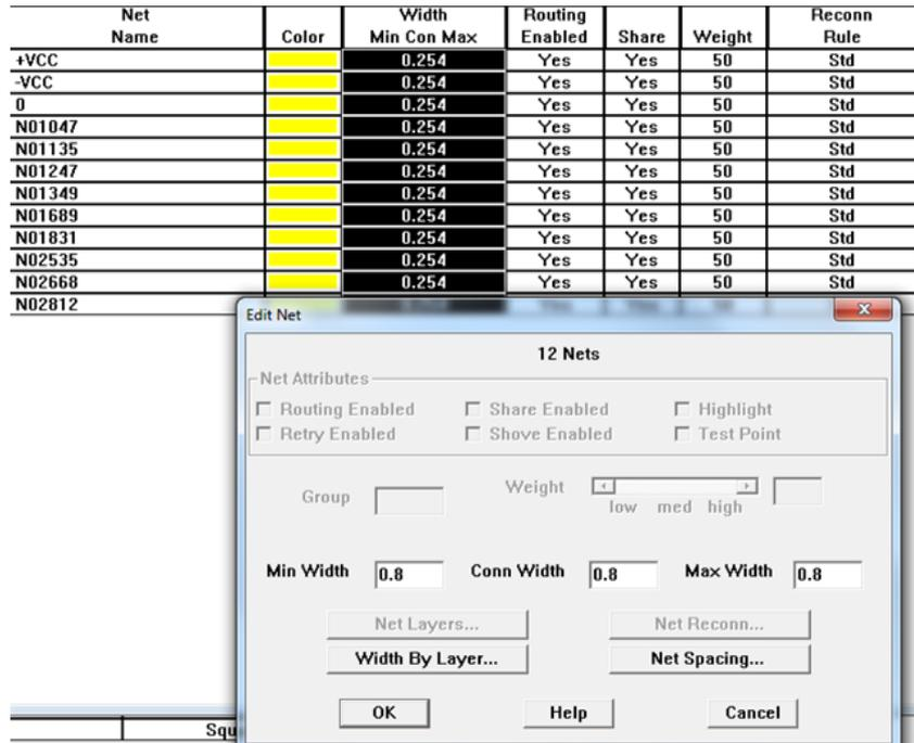
As it is our circuit, the spreadsheet is very simple. We can set the width individually for each track but, if all of them are to be equally wide we can click on the heading to select and modify all at once. The three parameters we encounter are set at 0,8 mm.
