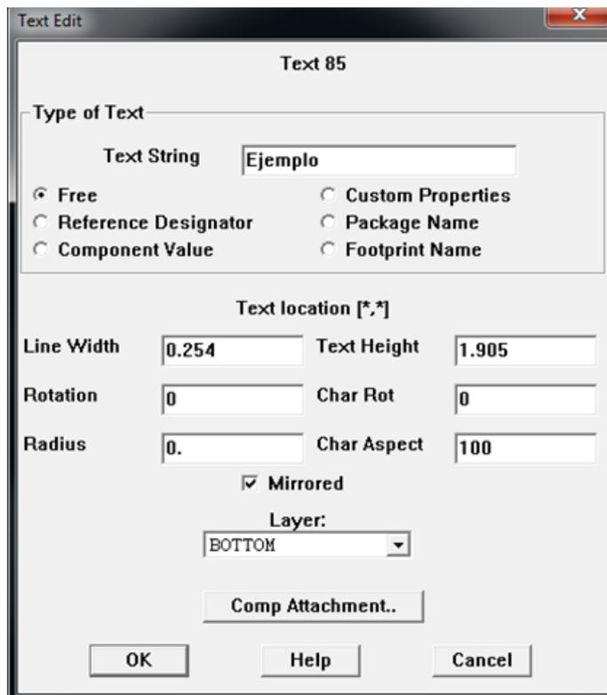
Size and width can be modified to fit the text into an available gap in the board. If the lines are too thin though, they may vanish during the etching process.
