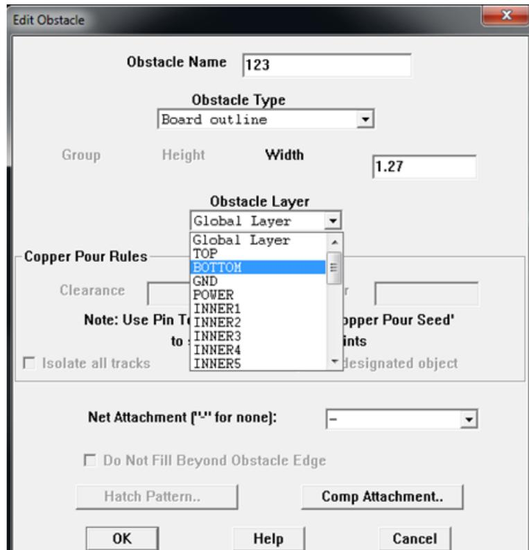
We will place it in the bottom layer since this will be the layer from which the design is to be transferred. Drawing this line is not intuitive unfortunately. Once again we have to remember that the usual “dragging” doesn’t work as expected in LAYOUT. We may need several attempts to come up with it.
