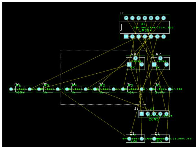
The dotted line represents the area where the design rules are checked. At this stage we recommend removing it by clicking on the DRC button.
