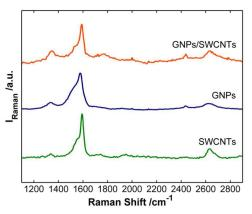
Fig. 4 Raman spectra of three electrodes fabricated, according to the proposed methodology, filtering the following dispersion volumes: 2 mL of GNPs (blue line), 0.5 mL of SWCNTs (green line) and, both consecutively, 2 mL of GNPs and 0.5 mL of SWCNTs (orange line).
