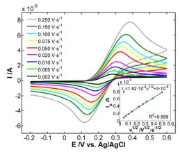
Fig. 8 Cyclic voltammograms of FcMeOH at different potential scan rates between 0.002 V s<sup>-1</sup> and 0.250 V s<sup>-1</sup>. Inset: Randles-Sevcik behaviour. Experimental conditions in text.
