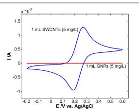
Fig. 5 Cyclic voltammograms obtained with two OTEs made of only GNPs or only SWCNTs. Experimental conditions in text.
