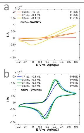
Fig. 7 Cyclic voltammograms of different GNPs/SWCNTs-OTEs (a) below percolation threshold of SWCNTs network, and (b) above percolation threshold of SWCNTs network. Experimental conditions in text.
