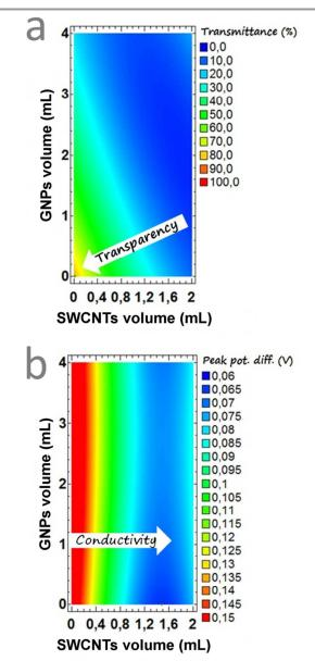
**Fig. 6** Response surfaces of the design of experiments for (a) transmittance of the GNPs/SWCNTs-OTEs at 550 nm, T<sub>550</sub>, and (b) peak potential difference,  $\Delta E_{\mu}$ , obtained in the cyclic voltammetry of FcMeOH, with respect to V<sub>GNPs</sub> and V<sub>SWCNTs</sub>. Experimental conditions in text.
