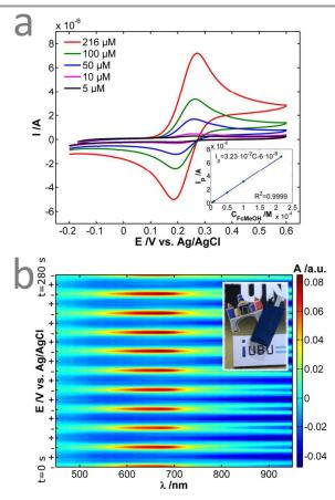
Fig. 9 (a) Cyclic voltammograms carried out with a GNPs/SWCNTs-OTE using FcMeOH concentrations ranged between 5 and 216  $\mu$ M. Inset: Calibration curve of FcMeOH. (b) 3D spectroelectrochemistry contour during ten consecutive doping/dedoping scans of PEDOT in a GNPs/SWCNTs-OTE. In the Y axis, "." is referred to a potential applied of -0.70 V and "+" to a potential applied of +0.70 V. Inset: The GNPs/SWCNTs-OTE modified with PEDOT by drop casting. Experimental conditions in text.
