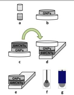
**Fig. 1** Fabrication process of GNPs/SWCNTs-OTEs: (a) preparation of the GNPs and SWCNTs dispersions, (b) filtration of the GNPs dispersion, (c) filtration of the SWCNTs dispersion, (d) press-transference of the bilayer film, (e) removing of the PTFE filter, (f) silver electrical contacts and (g) isolation of the silver electrical contacts.
