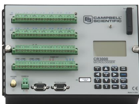
Figura 2.11: Datalogger Campbell Scientific CR-3000.
