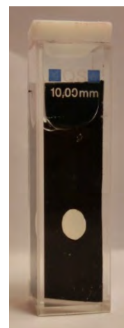
Figure 63. Cuvette adapted for measuring films.
