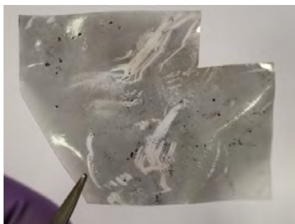
Figure 39. Picture of the polymer PB20_80A1 covered by Pd-NPs.
