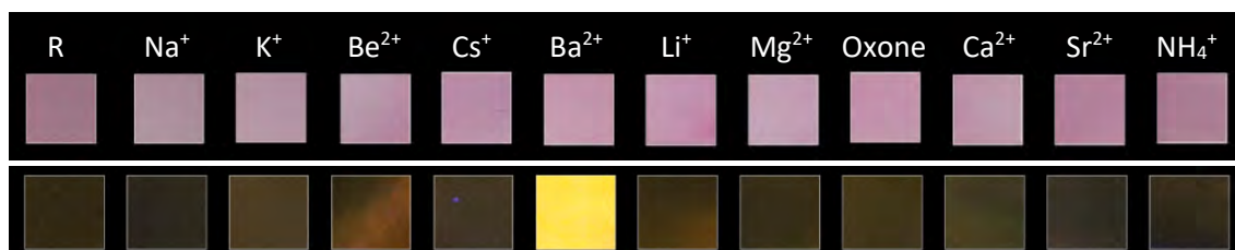
Figure 89. JG15dp in water, in the presence of different species (50 \mu M) under visible light (up) and under UV light (down). Ions sequence: Reference - Water- \text{Li}^+ - \text{Na}^+ - \text{K}^+ - \text{Rb}^+ - \text{Cs}^+ - \text{Mg}^{2+} - \text{Ca}^{2+} - \text{Sr}^{2+} - \text{Ba}^{2+} - \text{NH}_4^+ . Counterions: \text{ClO}_4^- , \text{CO}_3^{2-} ( \text{Cs}^+ ), \text{NO}_3^- ( \text{Rb}^+ )
