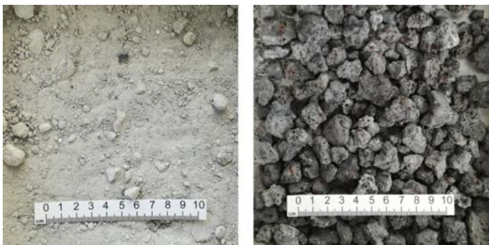
Fig. 1 – Ladle Furnace (LF) slag (left) and Electric Arc Furnace (EAF) slag (right) used in this research.
