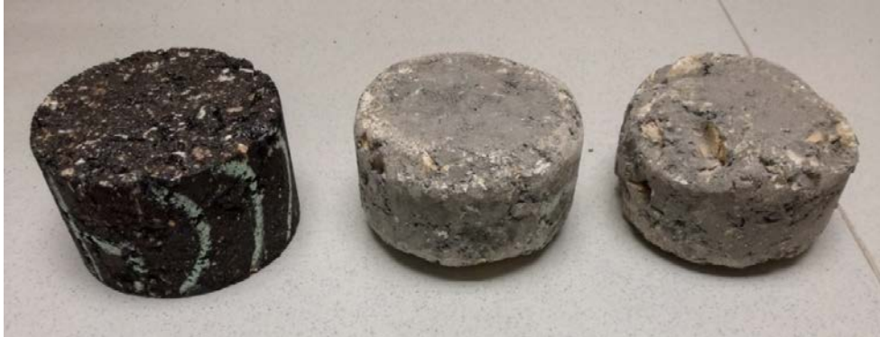
Fig. 4 – Specimens of the standard mix prior to testing, after the abrasion test and after the durability test (from left to right)
