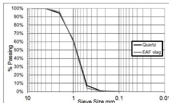
Fig. 1. Granulometry curve of the coating course aggregates.
