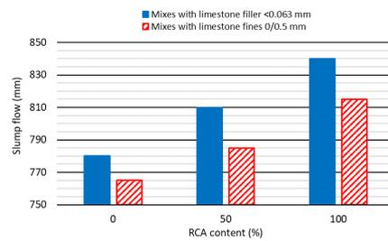
Fig. 2. Slump flow of the mixes.
