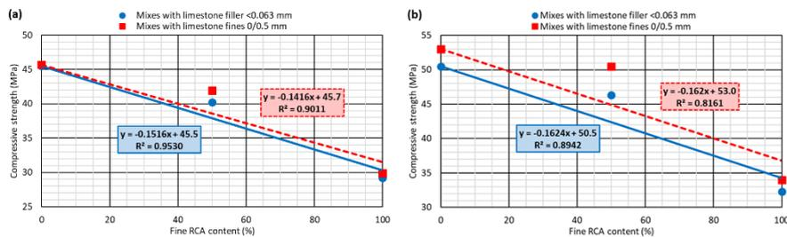
Fig. 3. Compressive strength at: (a) 7 days; (b) 28 days.
