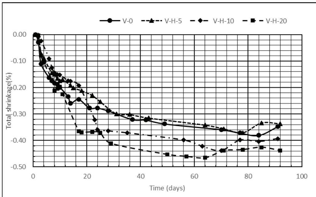
Fig. 4. Total shrinkage from 0 to 90 days.
