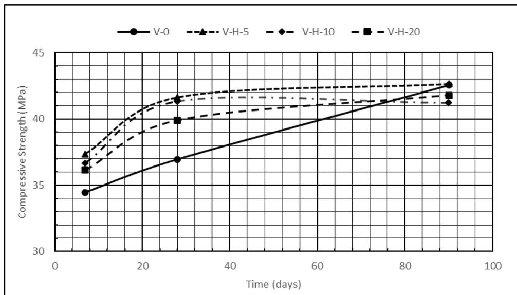
Fig. 2. Compressive strength at ages of 7, 28 and 90 days.
