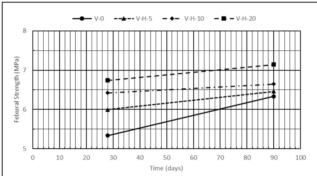
Fig. 3. Flexural strength at ages of 28 and 90 days.
