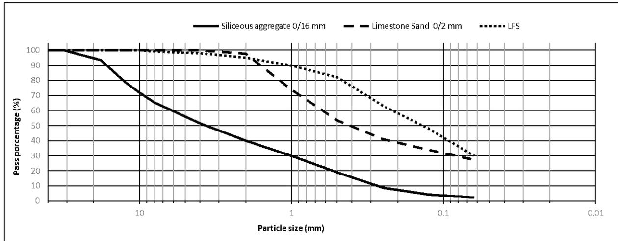
Figure 1. Particle gradation of the aggregates and LFS.
