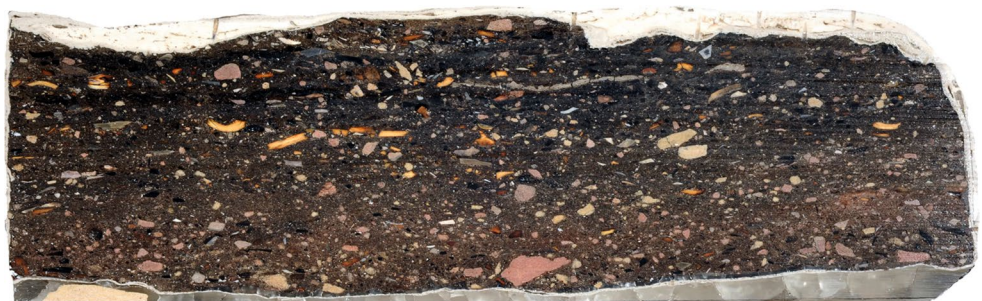
Fig. 19 A photo of an intact, resin-impregnated, 5 cm-thick slab with a clean profile. This slab was subsequently cut in half longitudinally and vertically: one half was then cut into thin sections and the other kept as a reference. Width of the block is ~70 cm
