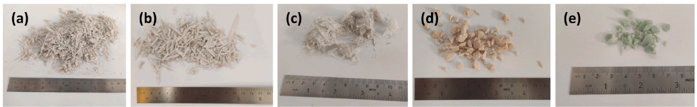
Fig. 2. WTBW: (a) overall material; (b) GFRP fibers; (c) GFRP microfibers; (d) balsa-wood particles; (e) polymeric particles.
