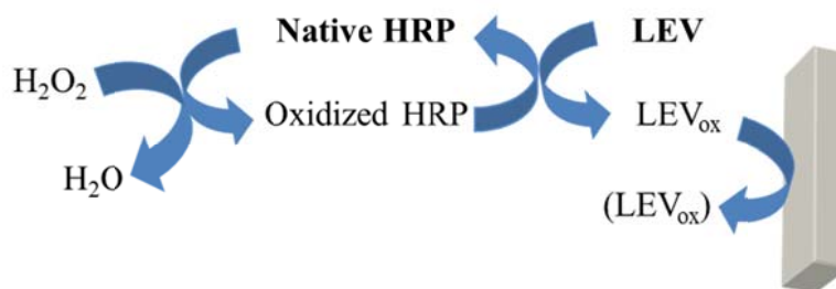
Figure 2.- Enzymatic mechanism for LEV determination
