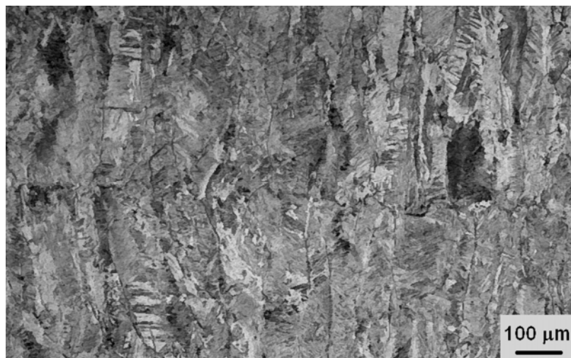
Fig. 2. Micrograph of the weld nugget of a RSW joint, which has a cast microstructure with coarse and columnar grains.
