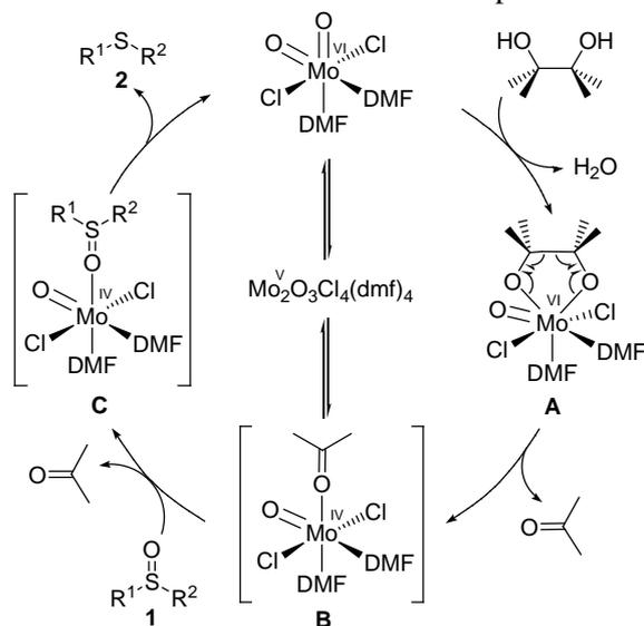
**Scheme 1.** Proposed catalytic cycle for the deoxygenation of sulfoxides with pinacol.
