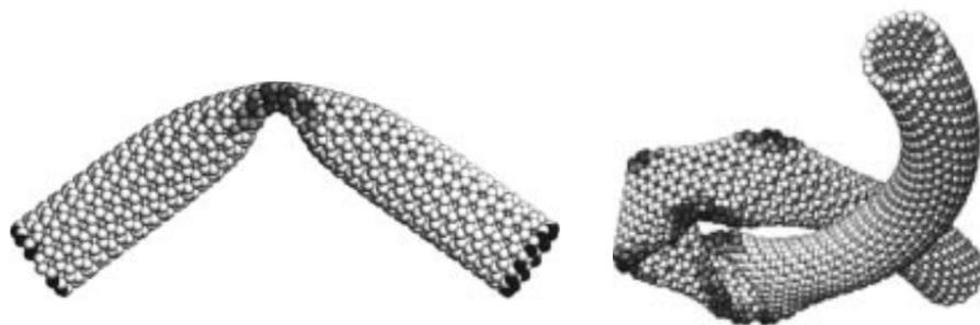
**Figure 2.32.** Theoretical CNT response to mechanical stress [210].
