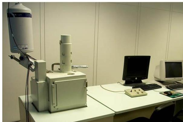
**Figure A-4.** JEOL JSM-6460LV Scanning Electron Microscope (adapted from [www.ubu.es.../meh](http://www.ubu.es.../meh)).
