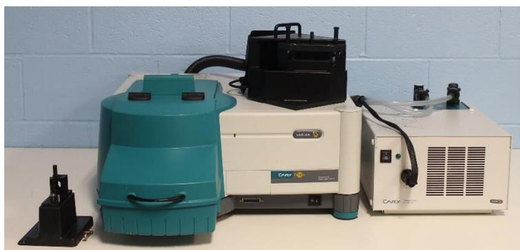
**Figure A-1.** Varian Cary Eclipse Fluorescence Spectrophotometer with Peltier-thermostated cell holder and temperature controller.
