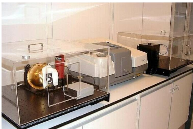
**Figure A-2.** FT-IR equipment (adapted from [www.ubu.es.../ft-ir](http://www.ubu.es.../ft-ir)).
