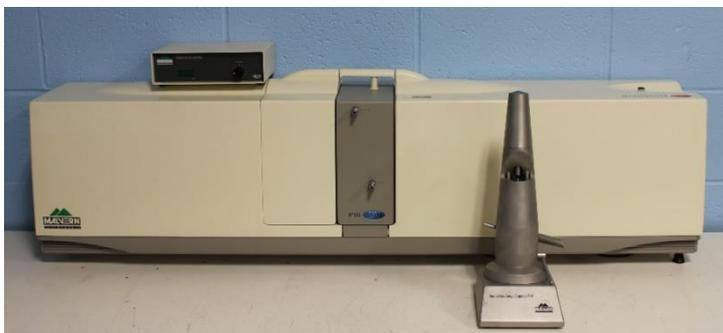
**Figure A- 12.** Malvern Mastersizer 2000 apparatus with Hydro 2000SM dispersion unit.
