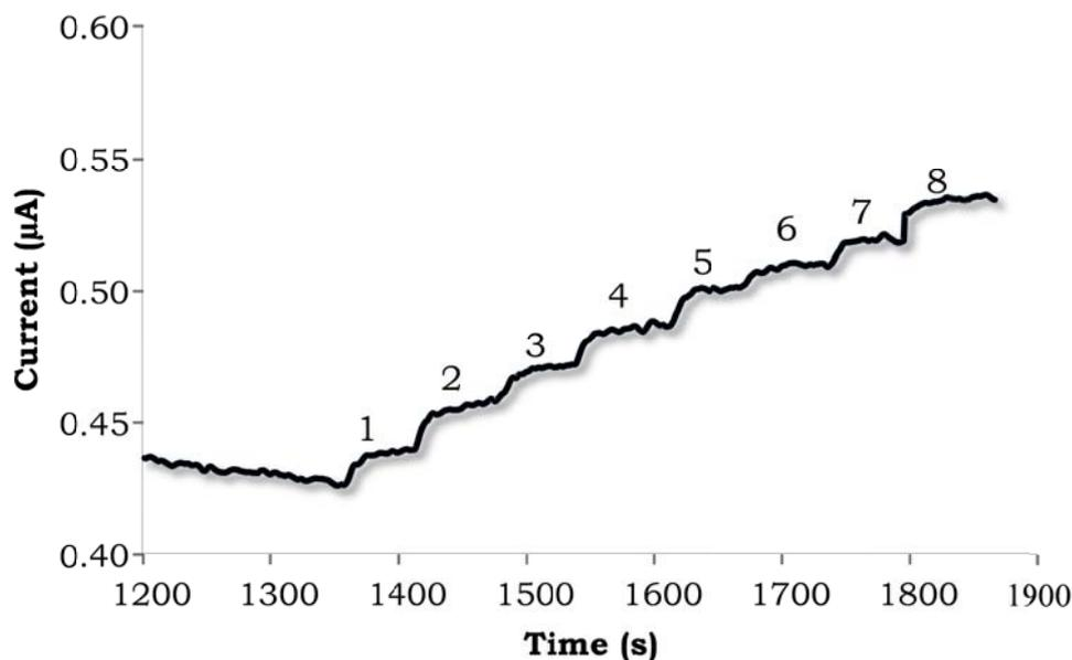
**Figure 6.3.** Chronoamperogram recorded for determination of Put using a PUO/TTF/SPCE based biosensor. 1-8, additions of 50  $\mu\text{L}$  of a 1 mM Put solution. pH, 10;  $E_{app}$ , + 300 mV vs Ag/AgCl- SPE
