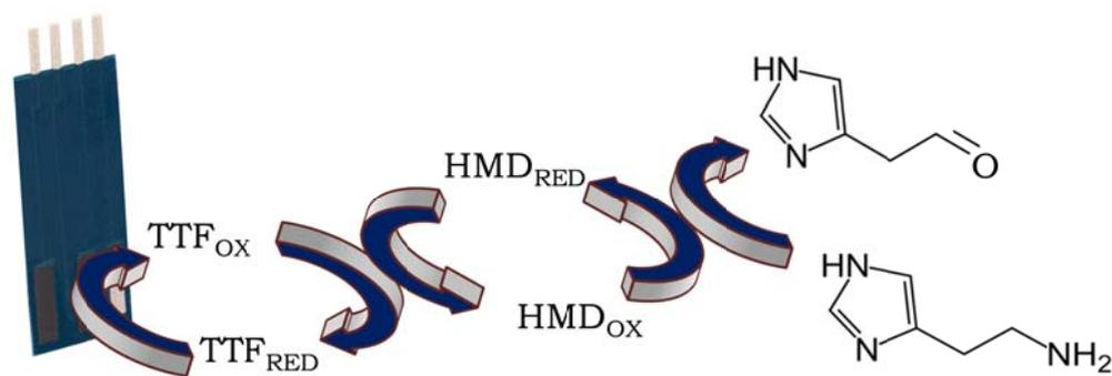
**Scheme 7.1.** Enzymatic mechanism of HMD/TTF/SPCEs biosensors
