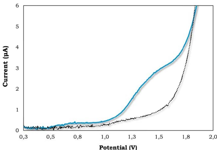
**Figure 8.2.** Square-wave voltammograms obtained using a BDD electrode in 10 mM  $\text{Na}_2\text{CO}_3$  and 100 mM  $\text{NaClO}_4$  (pH 10) for (---) blank and (—)  $[\text{His}] = 25 \mu\text{M}$ ;  $[\text{Cad}] = 25 \mu\text{M}$ ;  $[\text{Tyr}] = 25 \mu\text{M}$  and  $[\text{Put}] = 50 \mu\text{M}$ . Potentials vs Ag/AgCl reference electrode
