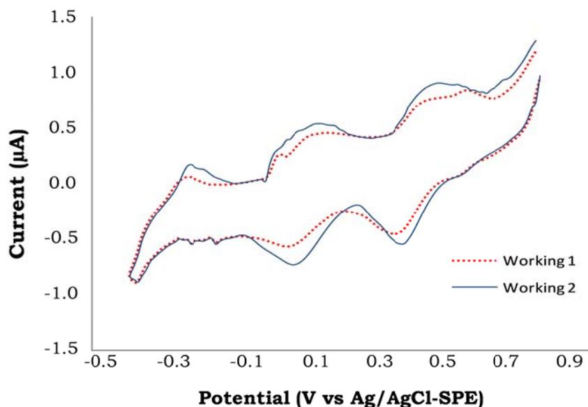
**Figure 5.3.** Cyclic voltammograms recorded in a 0.1 M KCl solution using an array-TTF/SPCE
