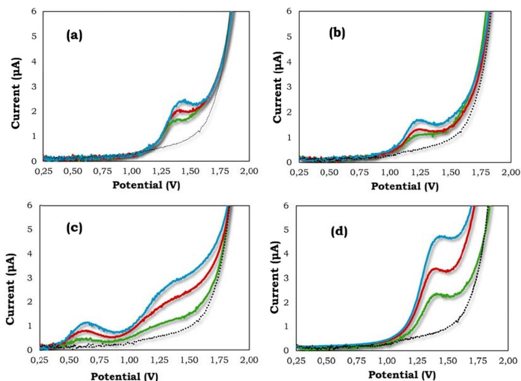
**Figure 8.1.** Square-wave voltammograms obtained using a BDD electrode in 10 mM  $\text{Na}_2\text{CO}_3$  and 100 mM  $\text{NaClO}_4$  (pH 10) for (···) 0; (—) 25; (—) 50 and (—) 75  $\mu\text{M}$  of (a) Put; (b) His; (c) Tyr and (d) Cad. Potentials vs Ag/AgCl reference electrode
