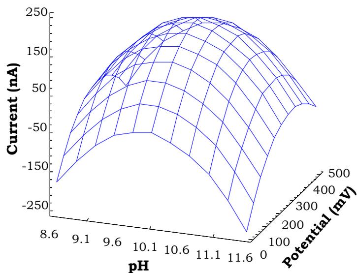
**Figure 6.4.** Response surface for the  $2^2$  central composite design performed for the optimization of the experimental variables for the analysis of Put using biosensor PUO/TTF/SPCEs
