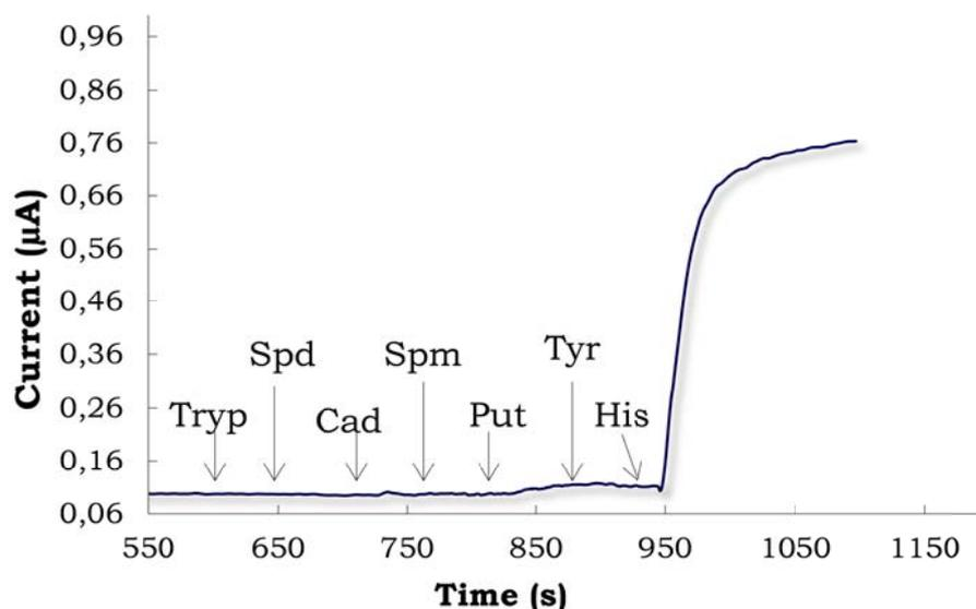
**Figure 7.3.** Chronoamperometric response obtained on HMD/TTF/SPCEs for different BAs at a 190  $\mu\text{M}$  concentration level (pH, 6.8; working potential, +130 mV vs Ag/AgCl SPE)
