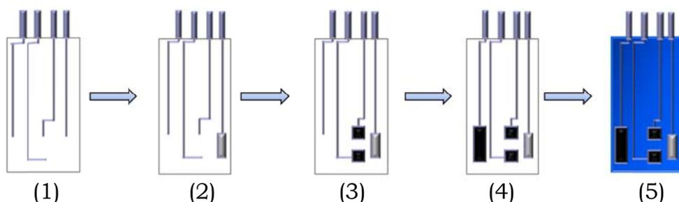
**Figure 5.2** Schematic diagram of the array-TTF/SPCEs preparation procedure: (1) Silver base-patterns, (2) reference electrode (Ag/AgCl), (3) working electrode (carbon ink + TTF 3 % with respect to the mass of the carbon ink), (4) counter electrode (carbon ink) and (5) insulator layer
