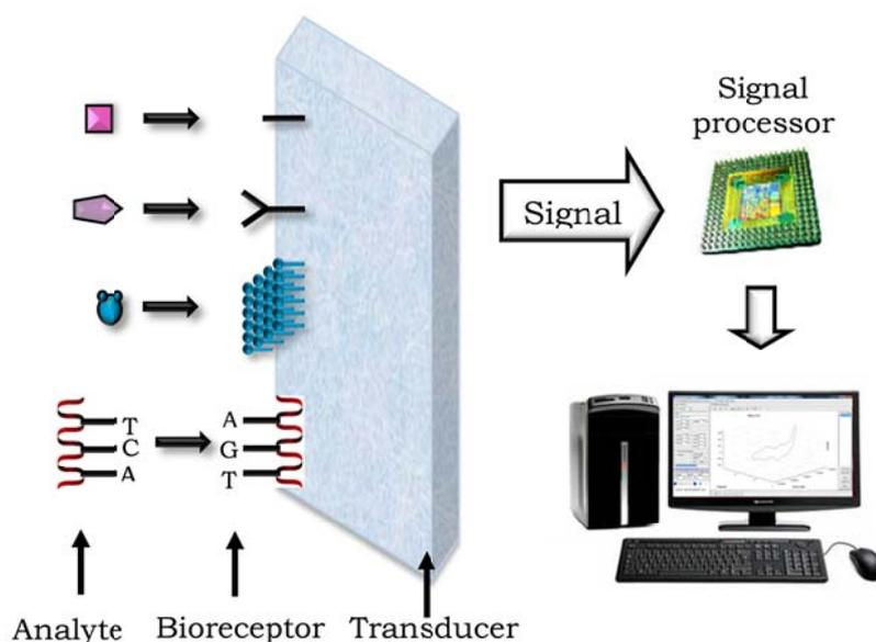
**Figure 3.1.** General scheme of a biosensor
