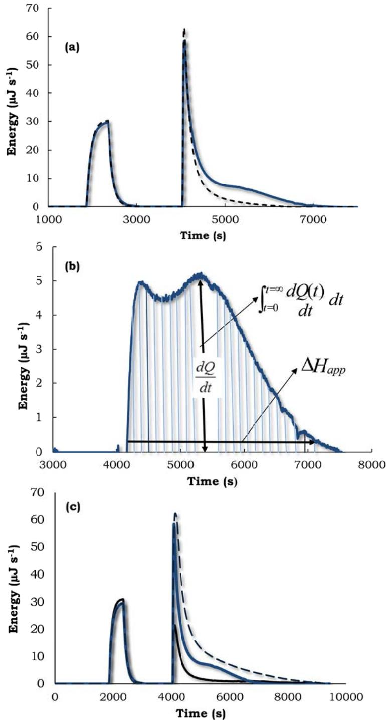
**Figure 6.1.** Thermal power registered for **(a)** a TTF/SPCE modified with BSA and GA (—) and a TTF/SPCE modified with PUO immobilized by crosslinking using BSA and GA (---). **(b)** Change in thermal power for PUO catalyzed oxidation of Put. Injections of 10 mL of Put 40 mM (4000 s) in phosphate buffer pH 10. **(c)** Thermal power registered using a PUO/TTF/SPCE for injections of 10 mL of Put (—), 25 mM (---) 40 mM and (- · -) 50 mM
