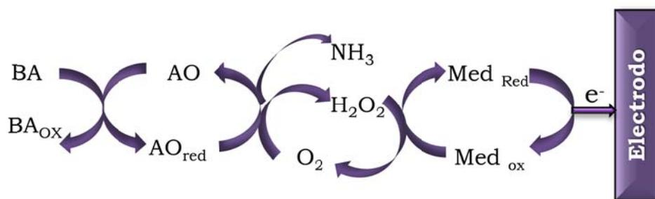
**Figure 3.17.** Mechanism of an AO based electrochemical biosensor using a redox mediator
