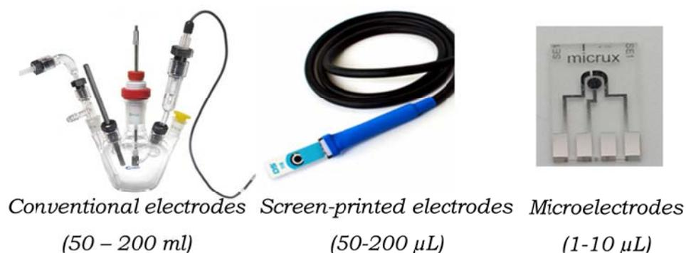
**Figure 3.12.** Miniaturization of the electrochemical electrodes
