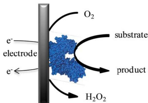
**Figure 3.9.** Schematic example of a first-generation biosensor
