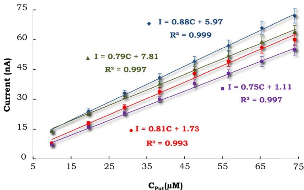
**Figure 6.5.** Experimental points and regressions for the different calibration curves carried out to evaluate the reproducibility in the determination of Put using PUO/TTF/SPCEs.
