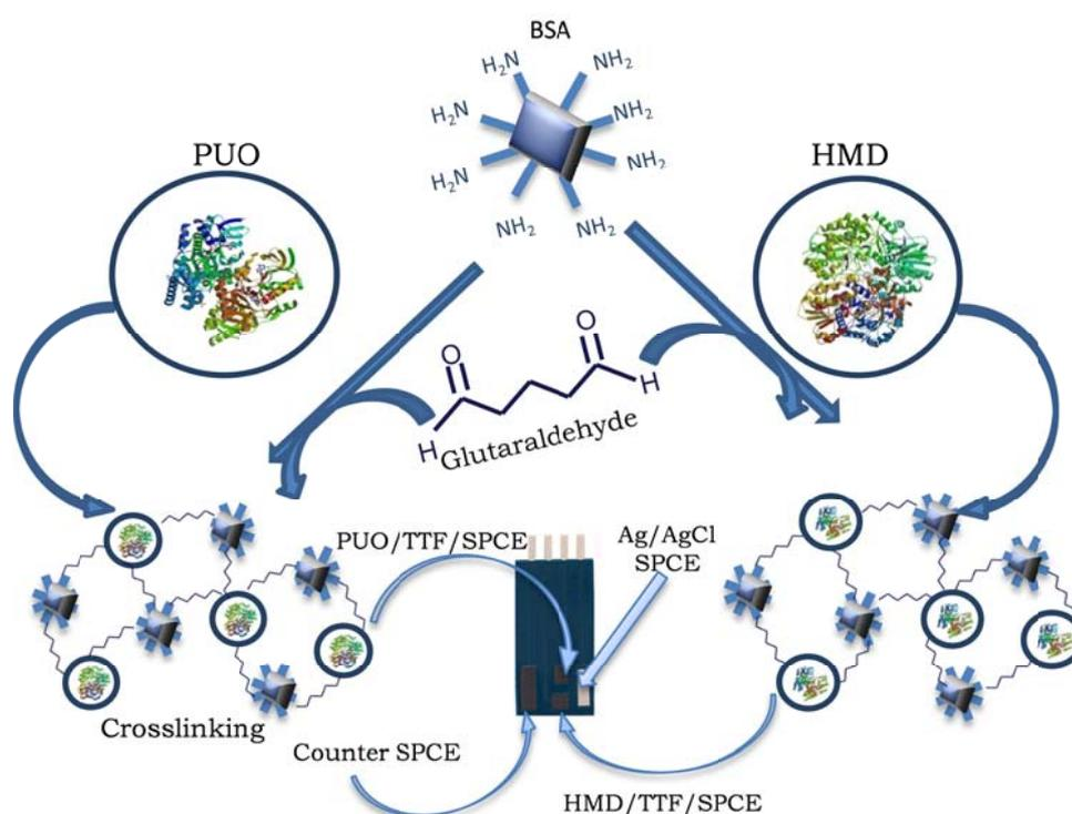
**Figure 7.1.** Scheme of a homemade dual-TTF/SPCE (1.3 cm x 2.8 cm)
