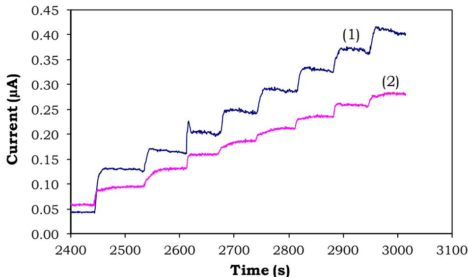
**Figure 5.4.** Chronoamperogram recorded for the simultaneous determination of Put and Cad in octopus samples in the array-TTF/SPCEs biosensor. (1) Working 1: MAO/TTF/SPCE and (2) working 2: MAO/AuNPs/TTF/SPCE. The first addition (2450 s) corresponds to 500 mL of sample extract and then successive additions of 100 mL of a 5 mM Put solution were made. pH 11,  $E_{ap} = +250$  mV vs. Ag/AgCl-SPE
