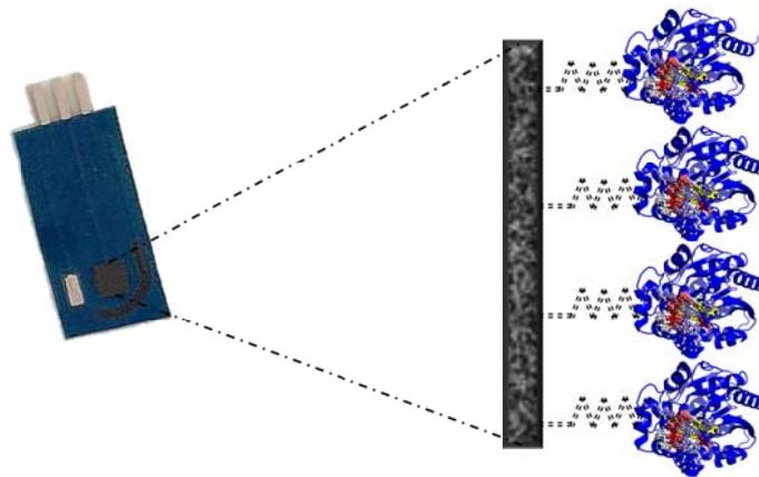
**Figure 3.6.** Schematic immobilization by covalent bonding
