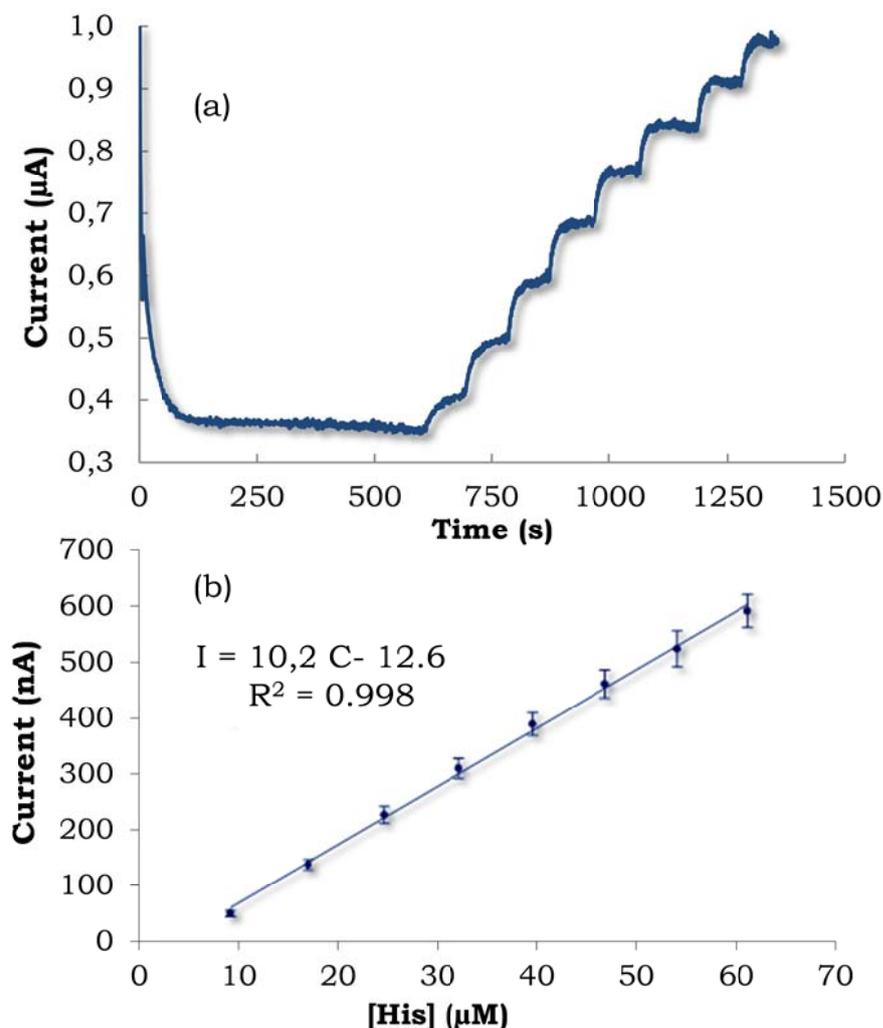
**Figure 7.2.** (a) Chronoamperogram recorded on HMD/TTF/SPCEs for successive additions of  $40 \mu\text{L}$  of a  $1 \text{ mM}$  His solution. (pH, 6.8; working potential, + 130 mV vs Ag/AgCl SPE). (b) Relation between amperometric current intensity and concentration of His in HMD/TTF/SPCEs biosensors (pH, 6.8; working potential, + 130 mV vs Ag/AgCl SPE)
