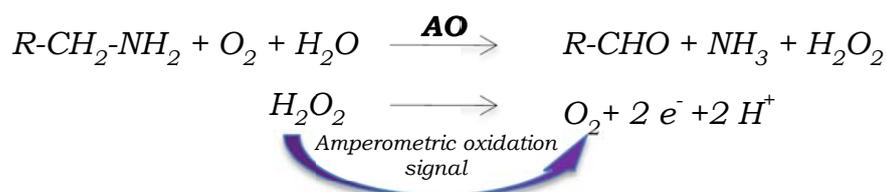
**Figure 3.16.** Mechanism of an AO based electrochemical biosensor
