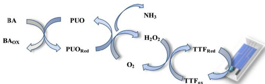
**Scheme 6.1.** Reaction occurring at surface of PUO/TTF/SPCEs biosensors during determination of Put
