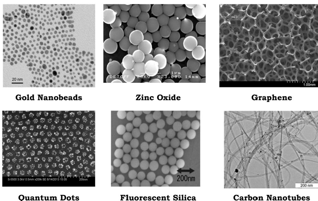
**Figure 3.8.** *Nanomaterials commonly applied in biosensor fabrication*
