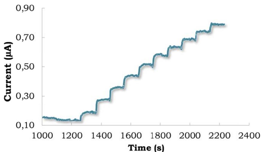
**Figure 4.2.** Chronoamperogram recorded for the determination of Put in anchovies samples using a MAO/TTF/SPCE based biosensor. The first addition (1300 s) corresponds to 100  $\mu\text{L}$  of sample extract and then successive additions of 50  $\mu\text{L}$  of a 1 mM Put solution were made
