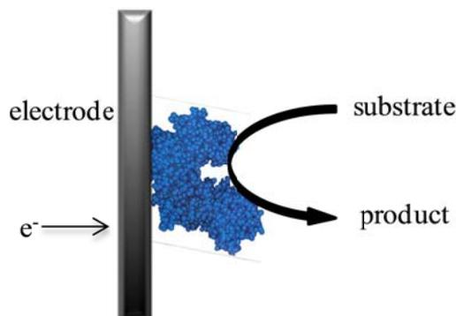
**Figure 3.11.** Schematic third-generation biosensor
