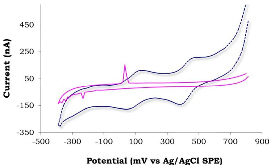
**Figure 4.1.** Cyclic voltammograms recorded in a 0.1 M KCl solution using a SPCE ( — ) and a TTF/SPCE (----). Scan rate; 0.1 V s<sup>-1</sup>
