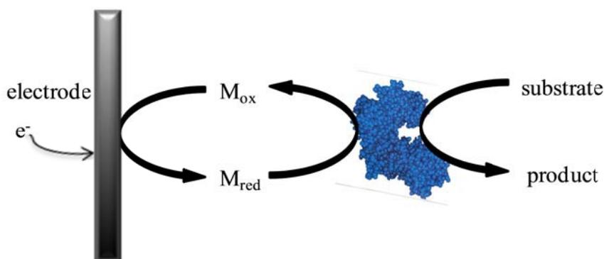
**Figure 3.10.** Schematic second-generation biosensor
