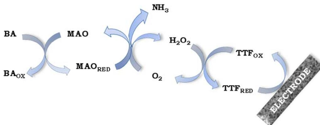
**Scheme 4.1.** Enzymatic mechanism of MAO/TTF/SPCEs biosensors
