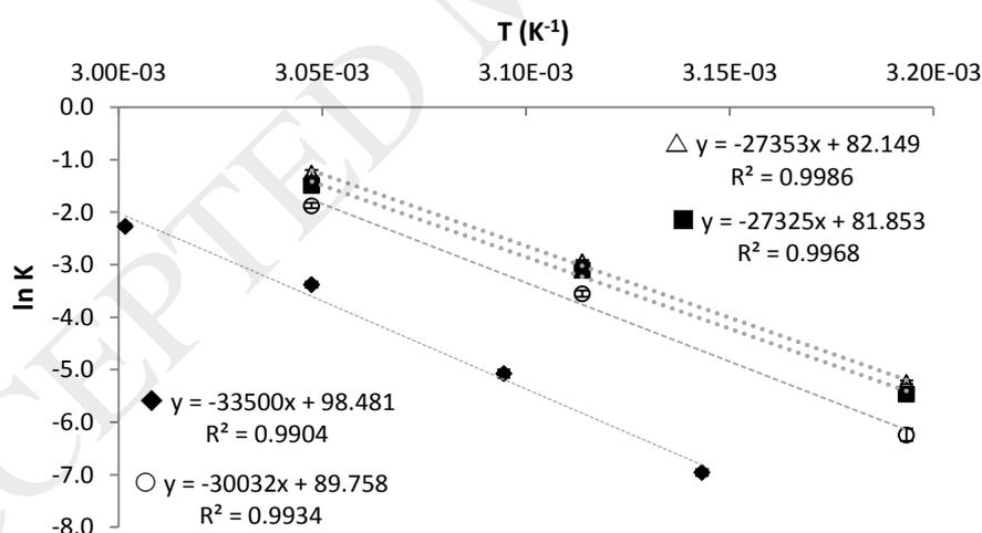
Figure 6. Temperature dependence of the kinetic constant used to calculate the activation energy at different pressures:  $\blacklozenge$  atmospheric pressure;  $\circ$  6 MPa;  $\blacksquare$  12 MPa and  $\triangle$  18 MPa.
