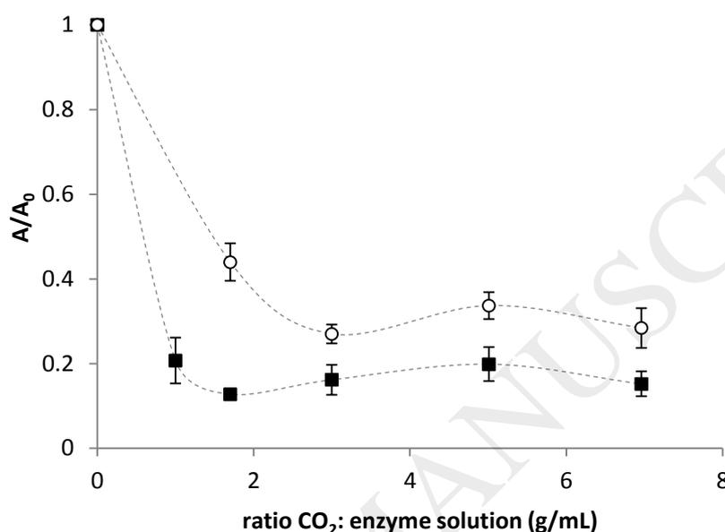
Figure 3. Residual activity of PME treated at 48 °C and 18 MPa for 15 (○) and 45 (■) minutes using different ratios  $\text{CO}_2$ :volume of enzyme solution.
