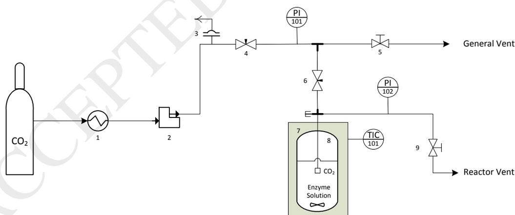
Figure 1. Experimental set-up of HPCD for inactivation of enzymes. 1: CO<sub>2</sub> cryostat; 2: Syringe pump (260D Teledyne ISCO); 3: bursting disk; 4: general process valve; 5: general vent valve; 6: individual inlet valve; 7: water bath; 8: high pressure batch reactor with magnetic stirring; 9: depressurization valve. PI-101: general pressure gauge; PI-102: reactor pressure gauge; TIC-101 temperature controller of water bath
