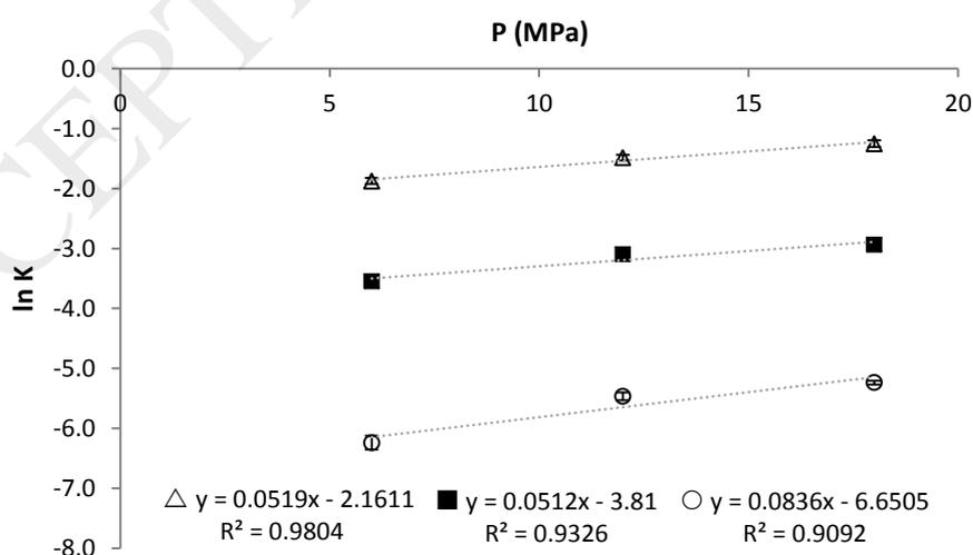
Figure 5. Pressure dependence of the kinetic constant used to calculate the activation volume at different temperatures: ○ 40 °C; ■ 48 °C and △ 55 °C.
