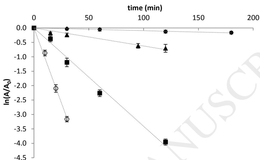
Figure 2. Inactivation of PME under atmospheric conditions at different temperatures: 45 °C (◆), 50 °C (▲), 55 °C (■) and 60 °C (○). The inactivation curves were modelled using a first-order model (dotted lines).
