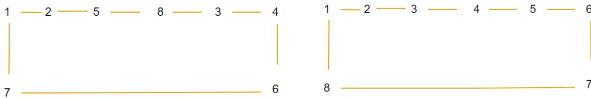
Figure 44. Proposed Power Grid Layouts: Shortest (Left) and Ring (Right)
