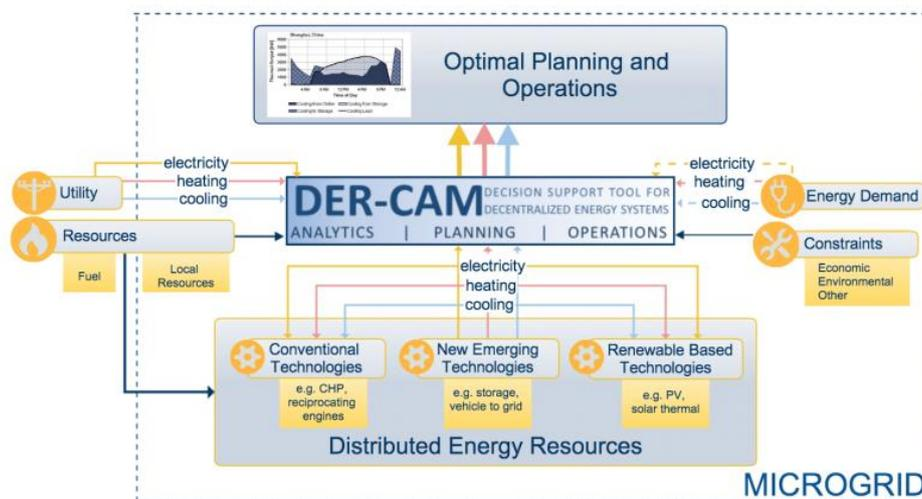
Figure 15. Inputs and Outputs by DER-CAM<sup>31</sup>
