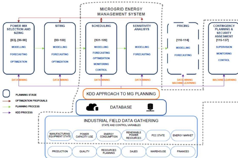
Fig. 3. A KDD-based approach to microgrid planning process scheme.
