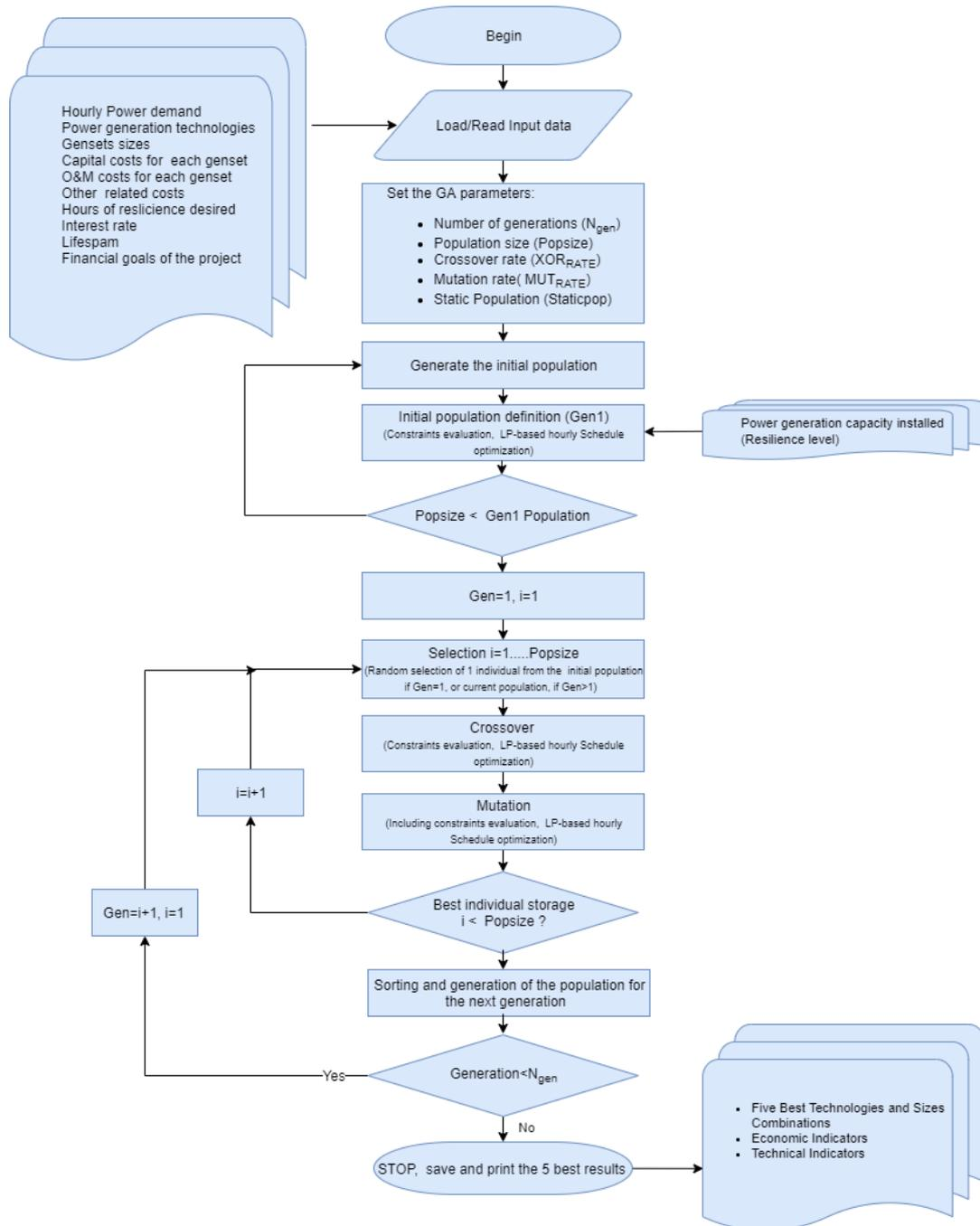
Figure 19. Flow Chart for the Genetic Algorithm Used for Power Lines Sizing, Siting and Scheduling
