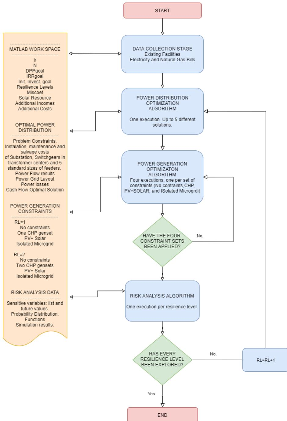
Figure 25. Sequence of Algorithms Executed in the Case Study
