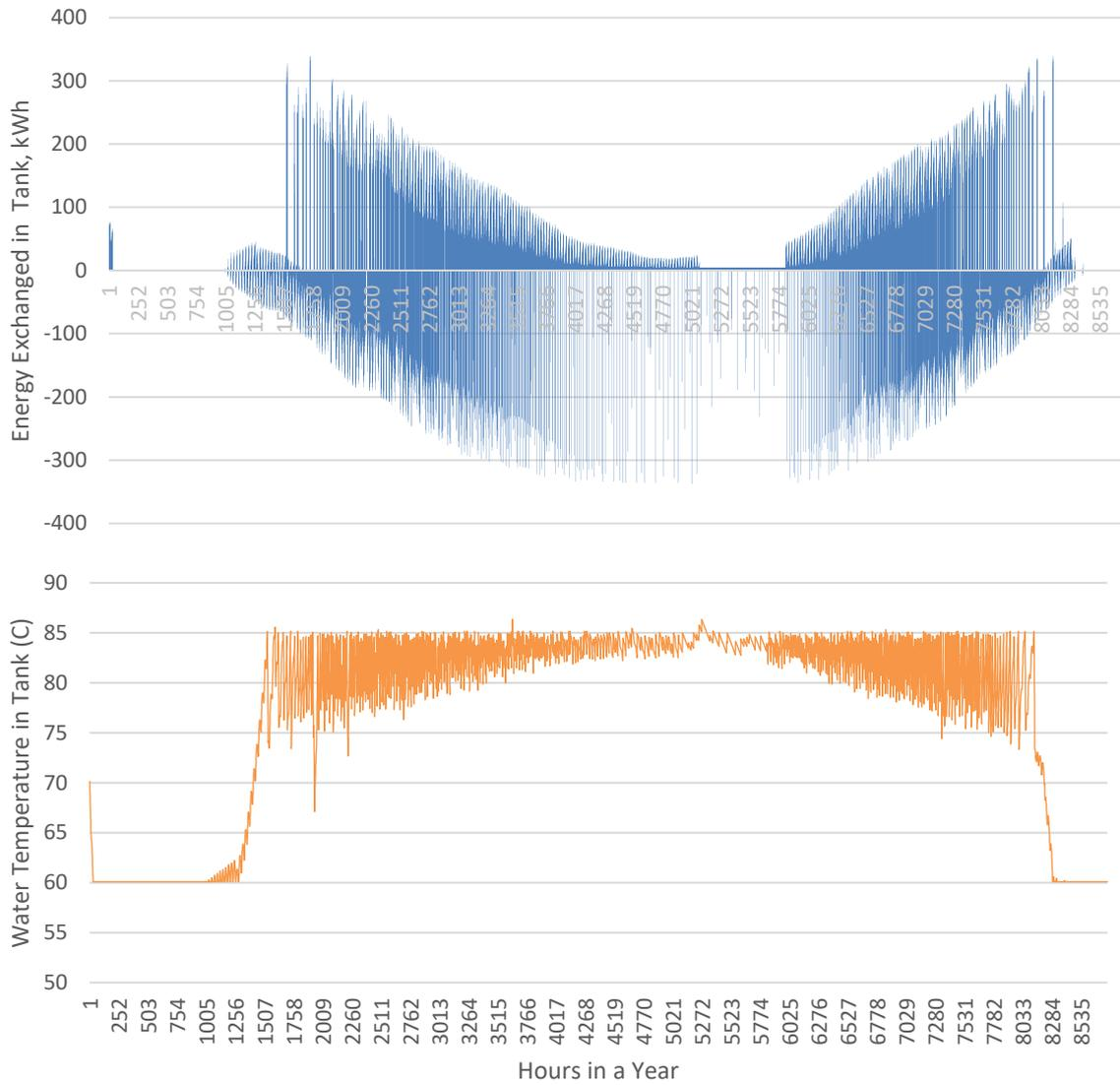
Figure 78 AP. Energy Exchanged in Tank and Water Temperature: Additional Resilience, Isolated Microgrid
