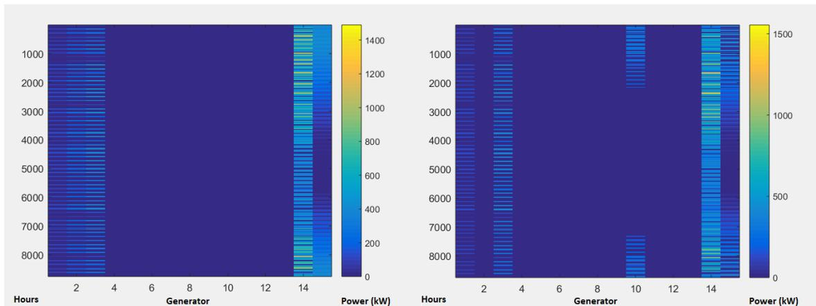
Figure 45. Generators per Solution and Scheduling for Customized Solutions 1 and 2. No Additional Resilience
