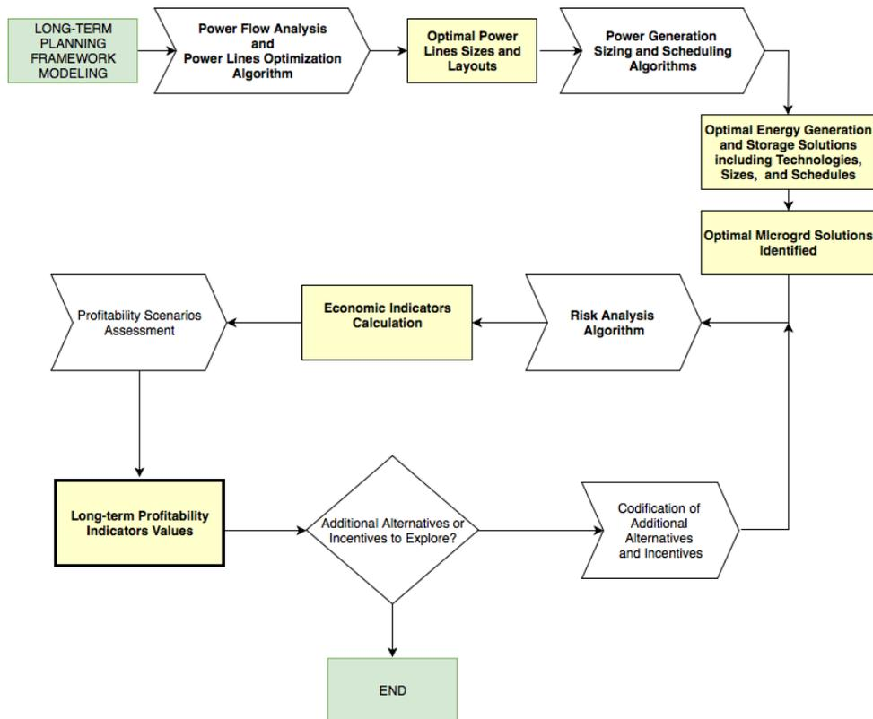
Figure 17. Algorithm Execution Sequence
