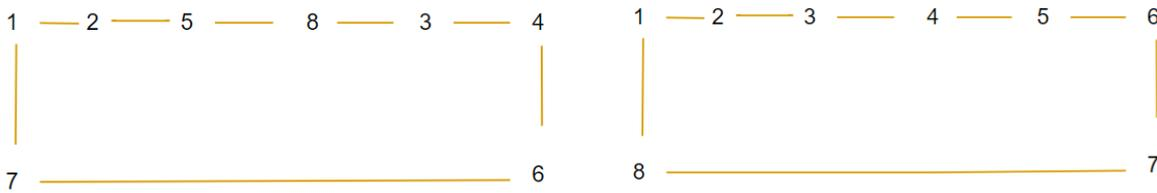
Figure AP68. Customized Power Grid Layouts: Shortest (Left) and Ring (Right)
