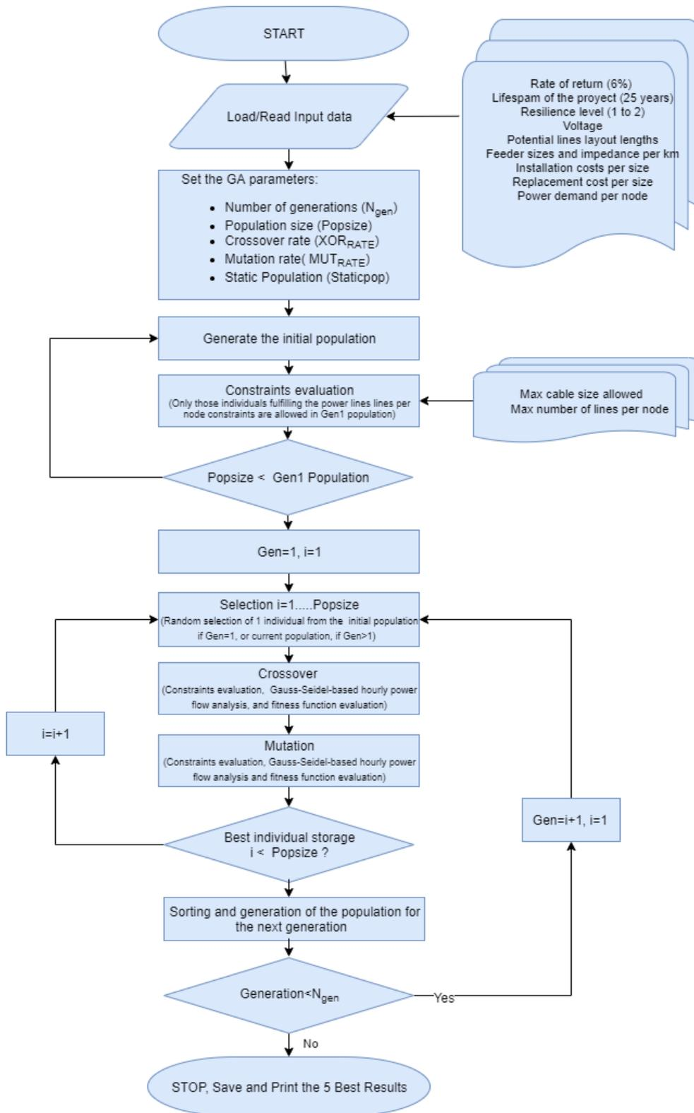
Figure 18. Flow Chart for the Genetic Algorithm used for the Selection, Sizing, and Scheduling of the Power Generation Systems.
