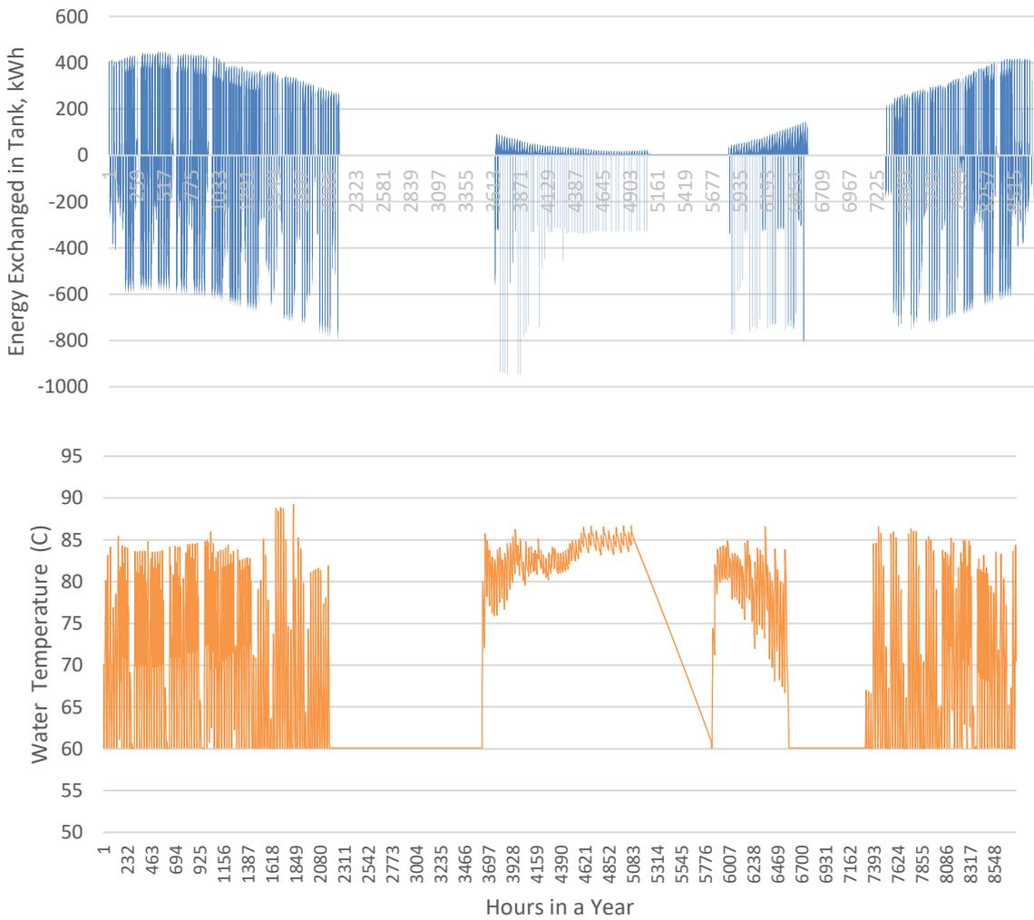
Figure 77 AP. Energy Exchanged in Tank and Water Temperature: Additional Resilience, Two CHP systems
