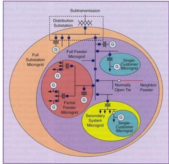
Figure 5. Future Power System Structure Source: IEEE Power & Energy. Vol.14, Number 5, September/October 2016
