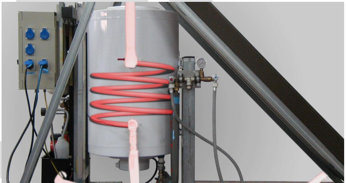
The storage system serves the purpose of storing heat transferred from the solar collector through the heat exchanger system.
