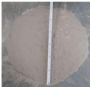
(a) Self-compacting concrete
