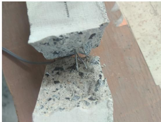
Fig. 6.5 Fibers crossing the cracking section
