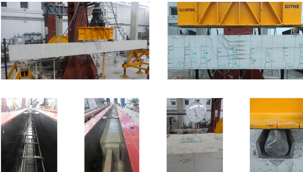
Fig. 7.14 Flexural beam set up
