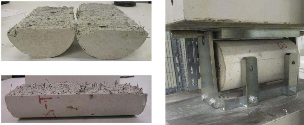
Fig. 5.4 Indirect tensile test
