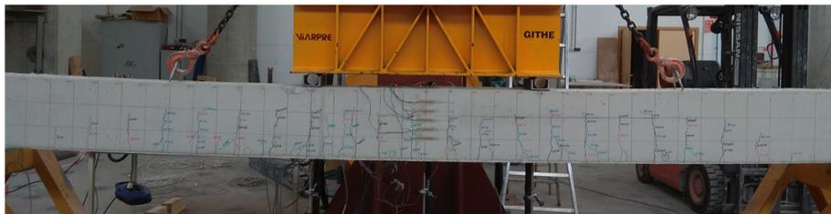
Fig. 7.16 Four-point bending beam tests
