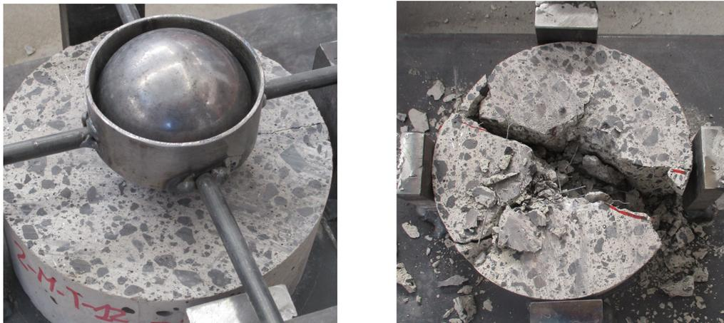
Fig. 5.12 Impact strength test
