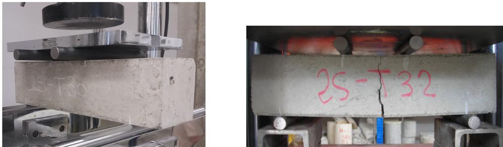
Fig. 5.6 Flexural test setup and failure
