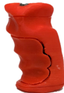
Pushbutton made by 3D scanning of a mold (photogrammetry).
