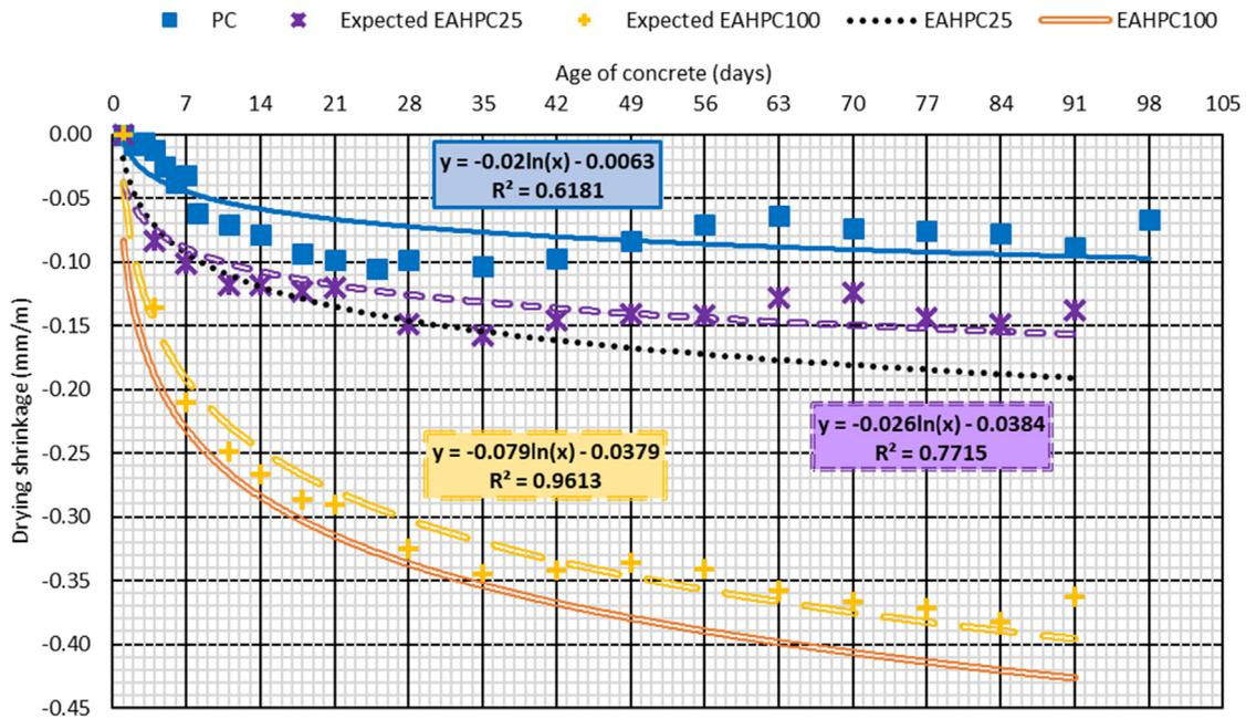
Fig. 16. Comparison between the expected and experimental drying shrinkage of the HPC mixes with early-age RA.
