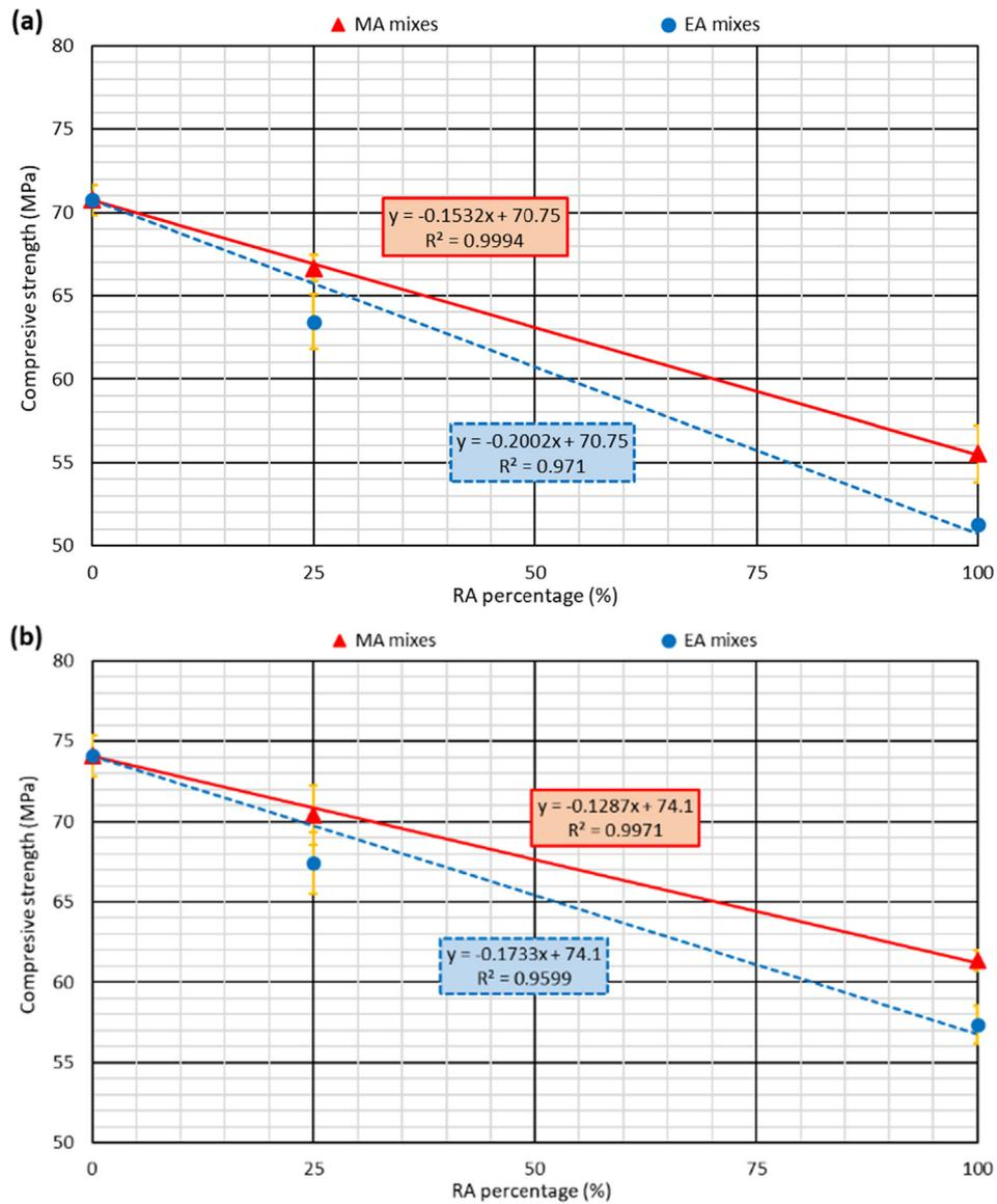
Fig. 9. Compressive strength of the mixes: (a) 7 days; (b) 28 days.
