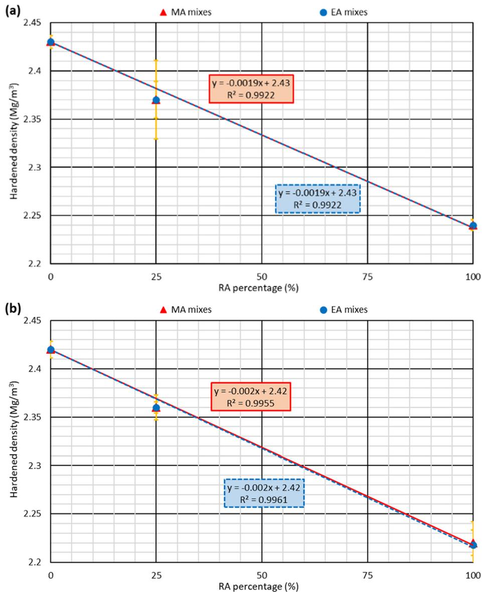
Fig. 7. Hardened density of the mixes: (a) at 7 days; (b) at 28 days.
