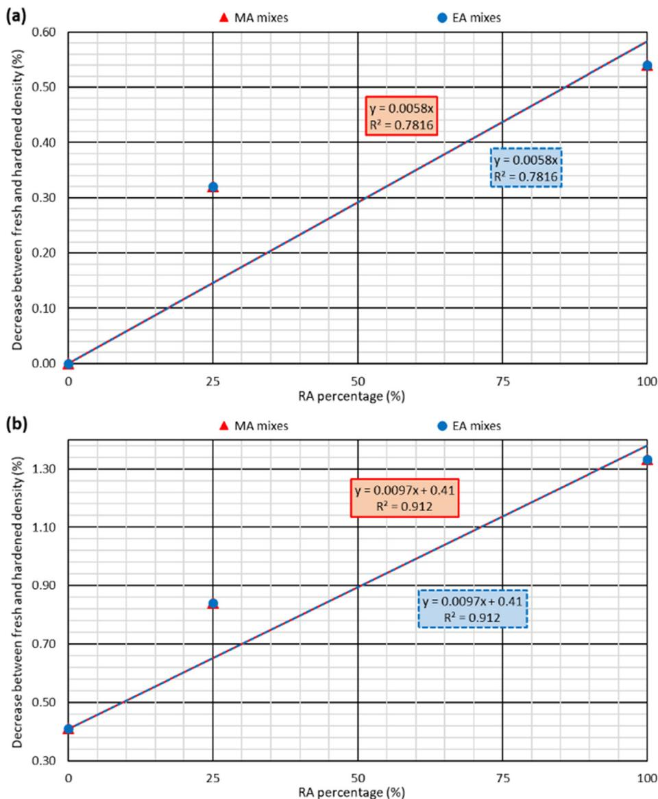
Fig. 8. Decrease between fresh and hardened density: (a) hardened density at 7 days; (b) hardened density at 28 days.
