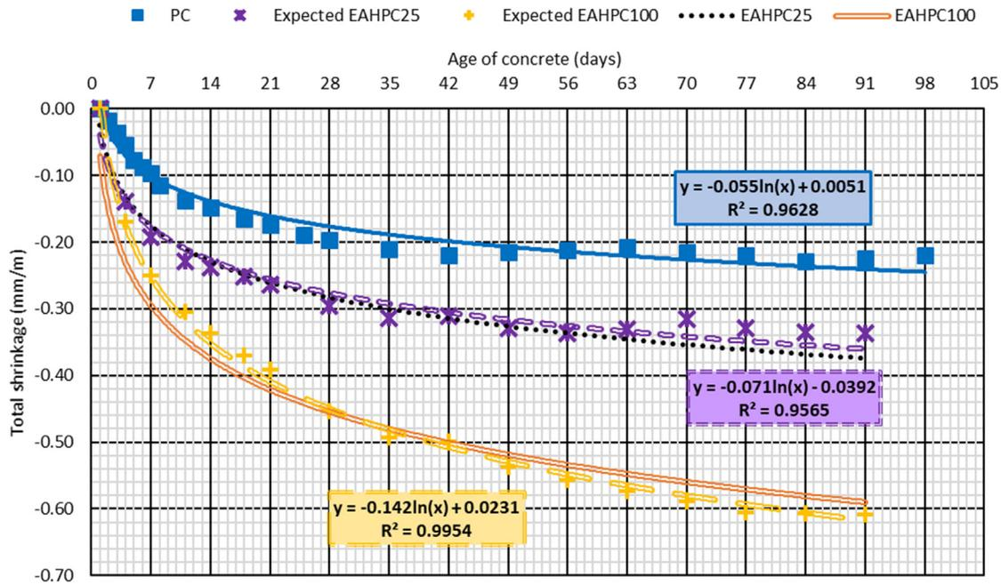
Fig. 18. Comparison between the expected and experimental total shrinkage of the HPC mixes with early-age RA.
