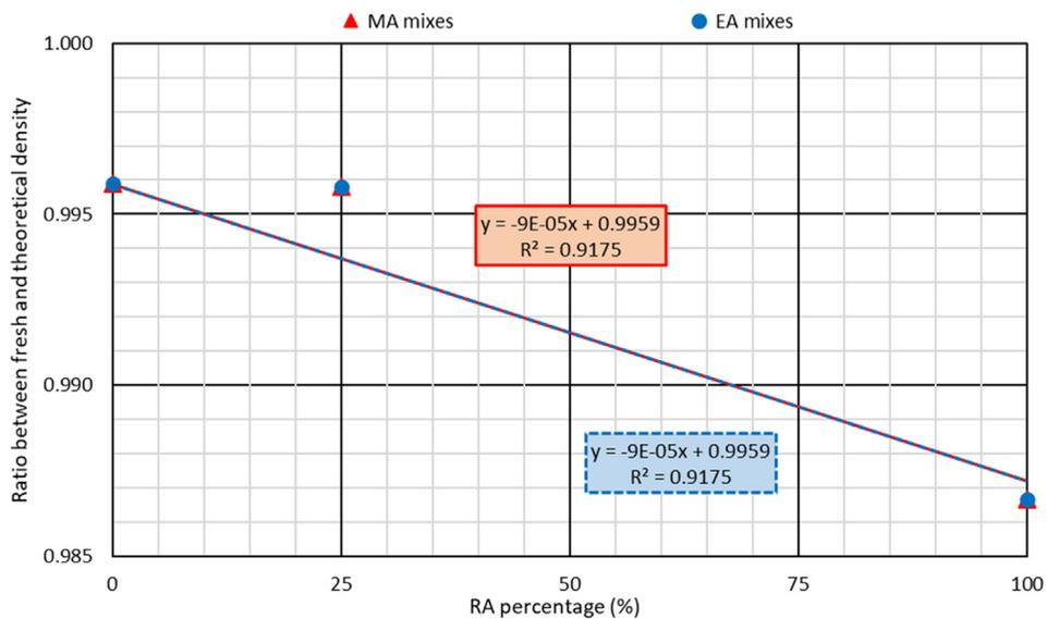
Fig. 6. Relationship between fresh and theoretical density of the mixes.
