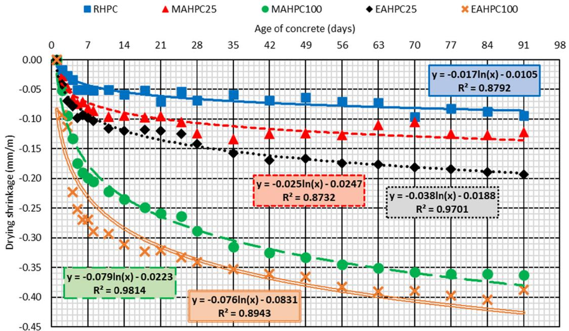
Fig. 15. Drying shrinkage of the mixes.
