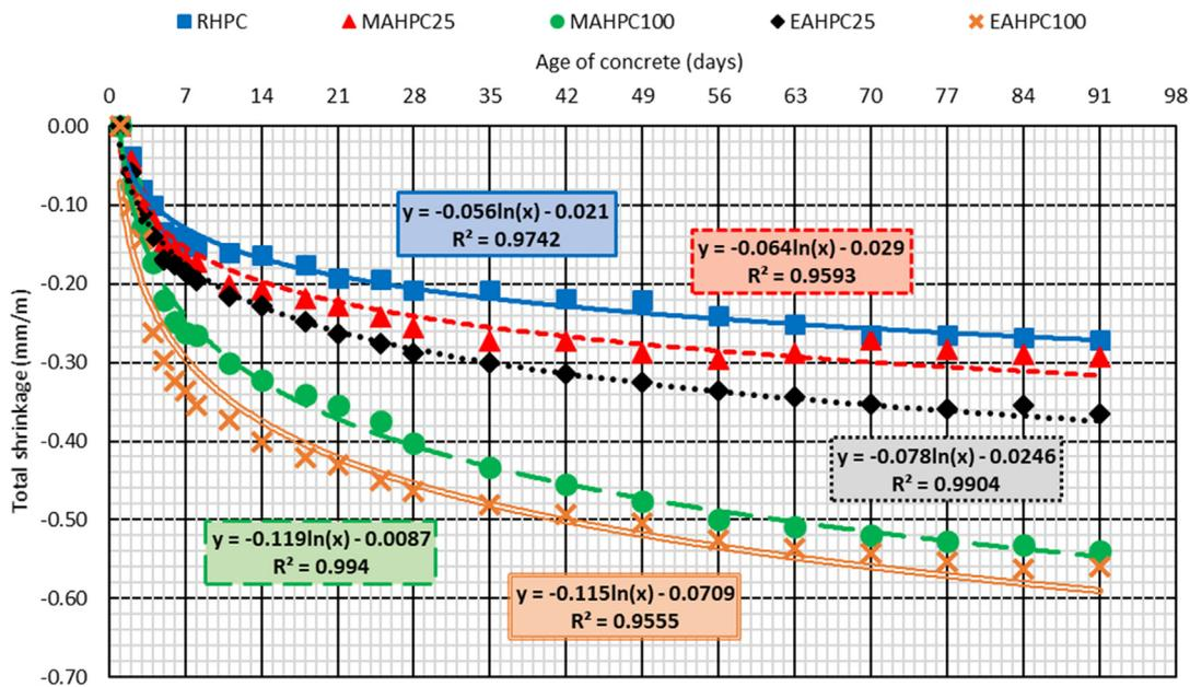
Fig. 17. Total shrinkage of the mixes.
