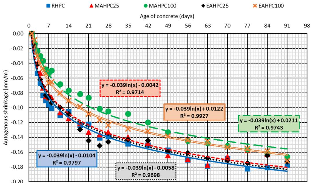
Fig. 13. Autogenous shrinkage of the mixes.
