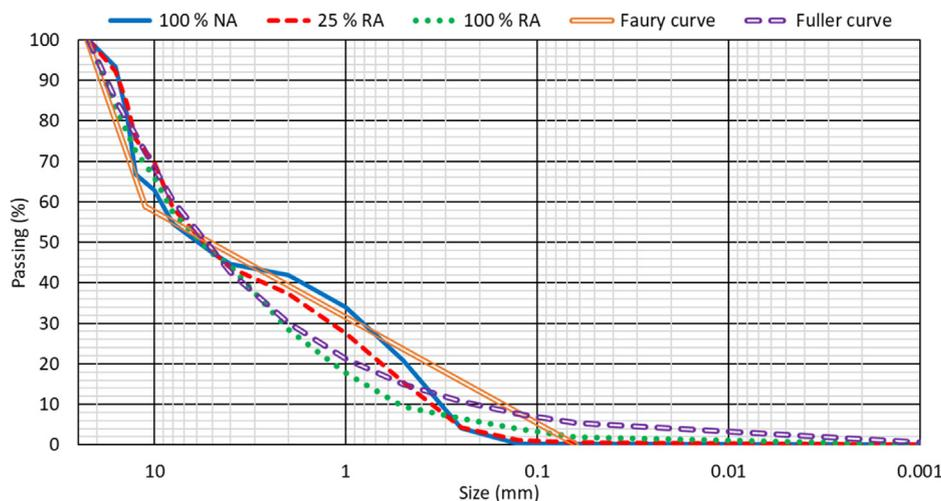
Fig. 2. Joint gradation of the mixes.
