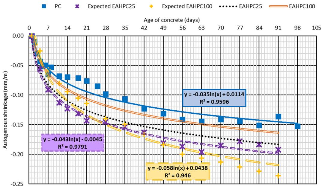
Fig. 14. Comparison between the expected and experimental autogenous shrinkage of the HPC mixes with early-age RA.
