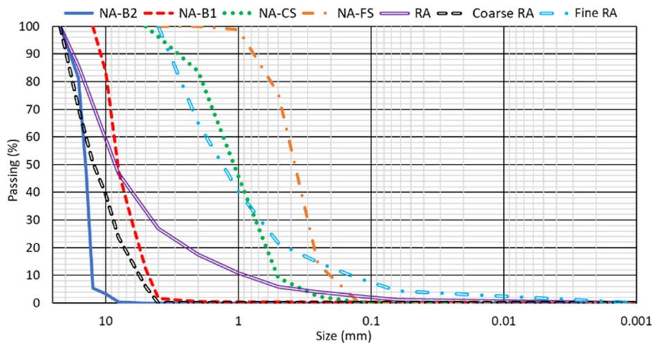
Fig. 1. Size distribution of the aggregates.
