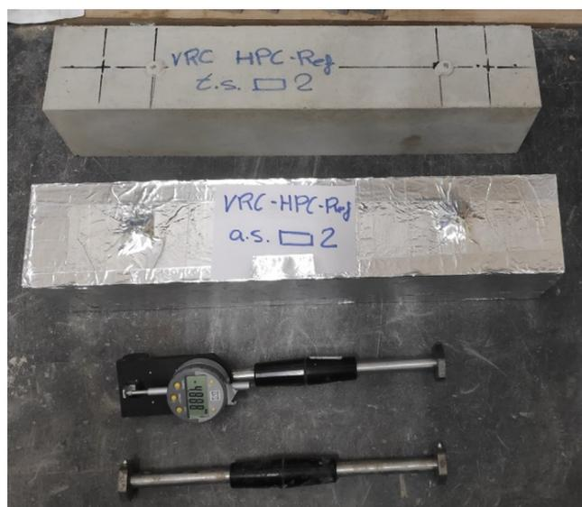
**Fig. 3.** Total-shrinkage specimen (up), autogenous-shrinkage specimen (in the middle), and shrinkage equipment (down).
