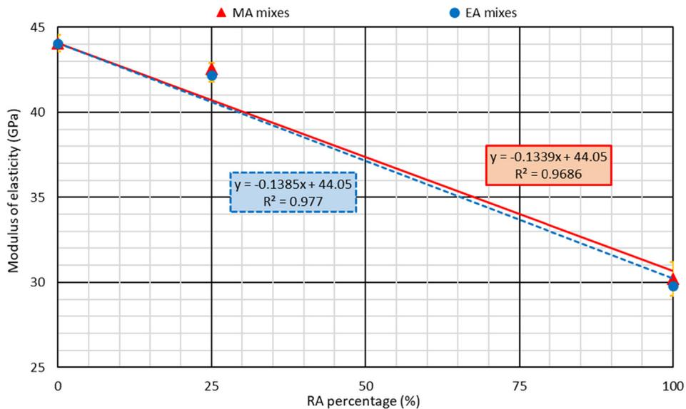
Fig. 11. Modulus of elasticity of the mixes at 28 days.
