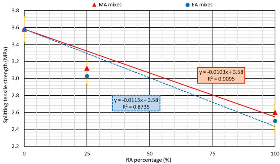
Fig. 10. Splitting tensile strength of the mixes at 28 days.
