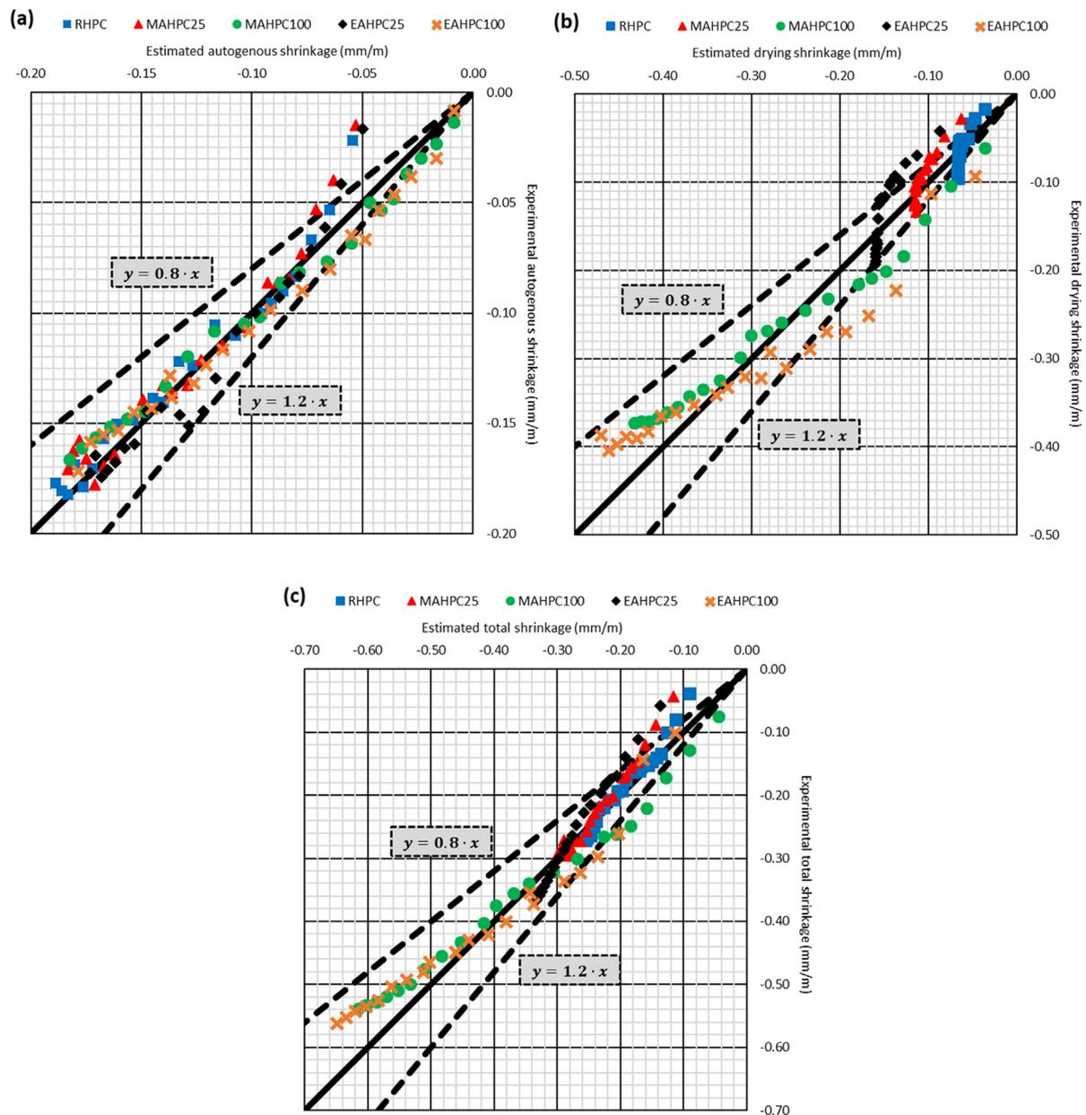
**Fig. 19.** Comparison between experimental and predicted shrinkage according to the model developed: (a) autogenous shrinkage; (b) drying shrinkage; (c) total shrinkage.
