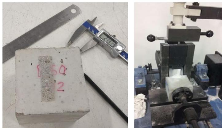
Figure 2.19. Abrasion test. Left: footprint on the M50 mix. Right: sample set up in the testing machine
