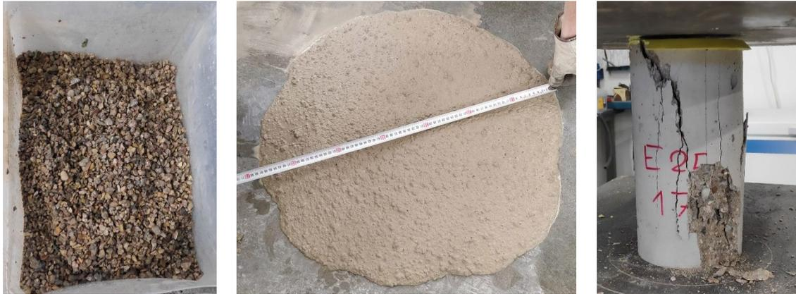
**Figure 3.2.** Highlights of the experimental plan: coarse RCA pre-soaked (left), slump-flow test of mix SA50 (middle), and specimen tested for compressive strength (right)
