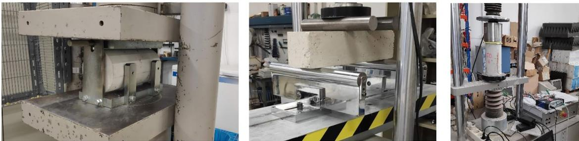
Figure 2.5. Mechanical tests: splitting tensile strength (left); flexural strength (middle); modulus of elasticity (right)
