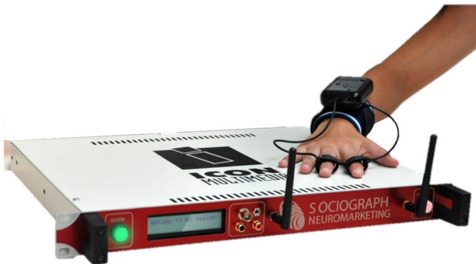
Figure 13: The electrodermal remote device (Sociograph® Technology) is wrapped around the left forearm, connecting two diodes at the 2nd and 3rd fingertips, and recording both tonic and phasic activity.
