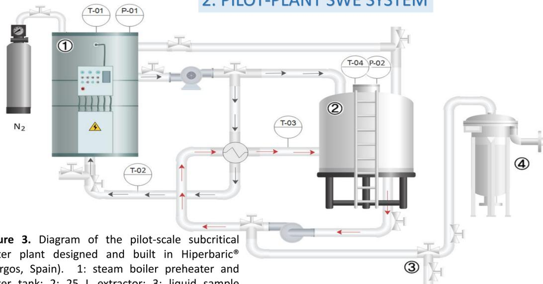
Figure 3. Diagram of the pilot-scale subcritical water plant designed and built in Hiperbaric® (Burgos, Spain). 1: steam boiler preheater and water tank; 2: 25 L extractor; 3: liquid sample collector; 4: filtration tank.
