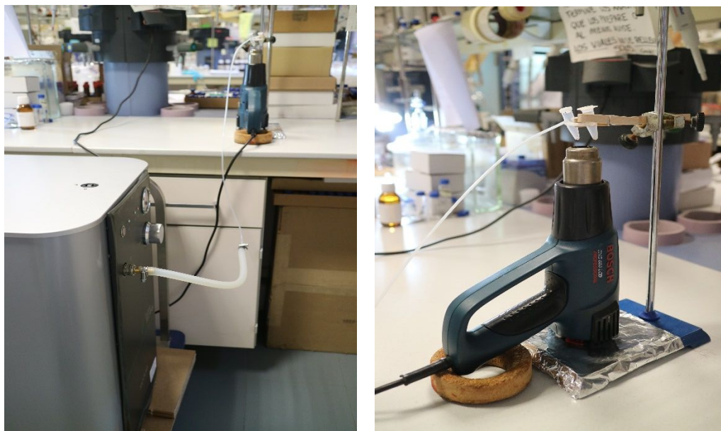
Figure S6. Complete recirculation system (left) designed for the experiment and close up view (right).
