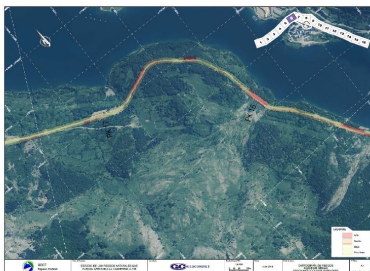
Fig. 12 - Map of a sector of the A-136 road classified with RHRS (Geoconsult, 2018).
