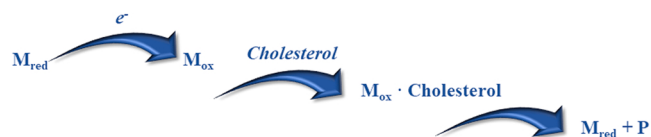
Fig. 4. Scheme of the indirect oxidation of cholesterol in presence of redox mediators.
