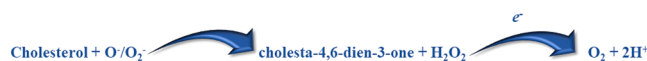
Fig. 7. Schematic of oxidation of cholesterol through the oxidation of H 2 O 2 at the electrode surface.
