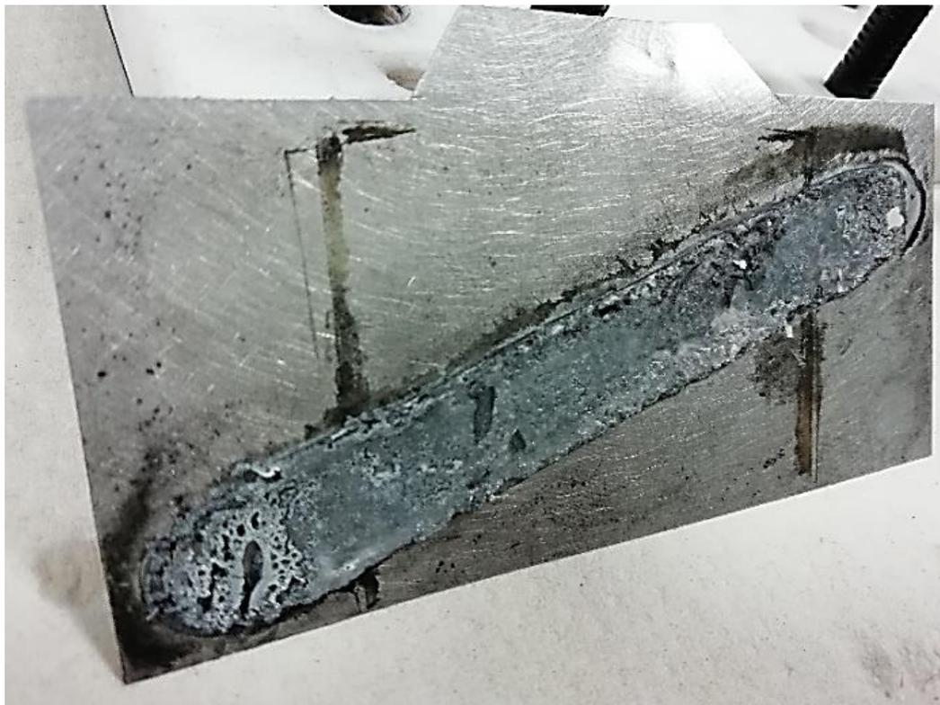
*Figure 5 - 5 Photograph of the negative zinc electrode after 500 cycles.*
