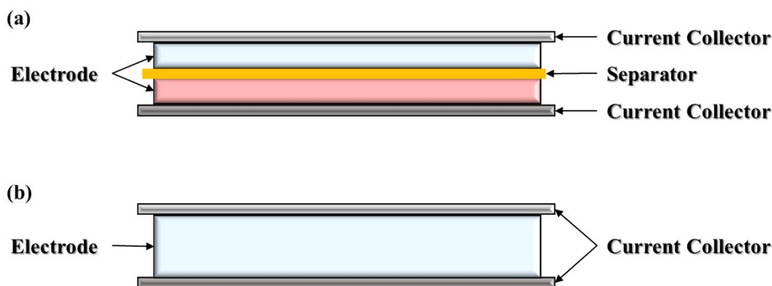
*Figure 3 - 2. Cell design for (a) Conventional battery and (b) Separator-free configuration for determination of electrical properties of semi-solid electrodes.*
