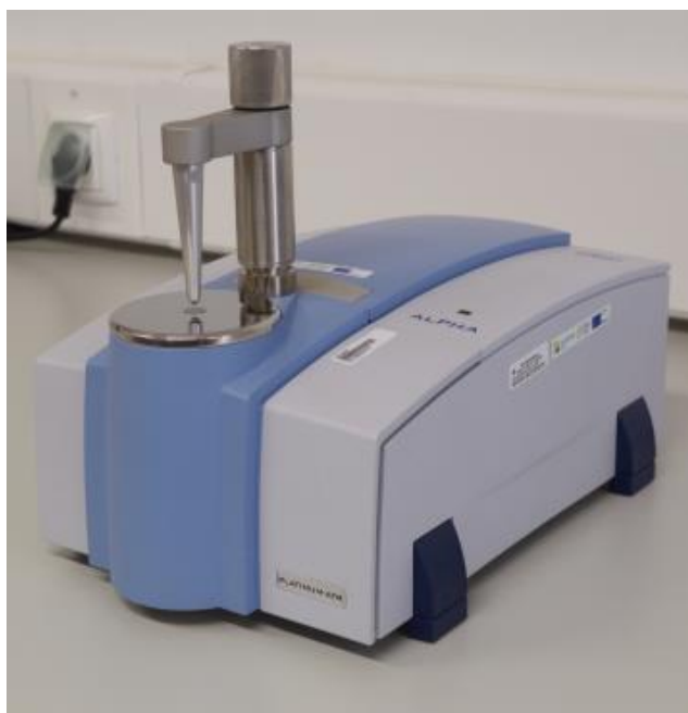
Fig. 3.11: Fourier Transform Infrared Spectroscopy utilized in this thesis investigation. © HERCULES Laboratory, University of Évora, Portugal.
