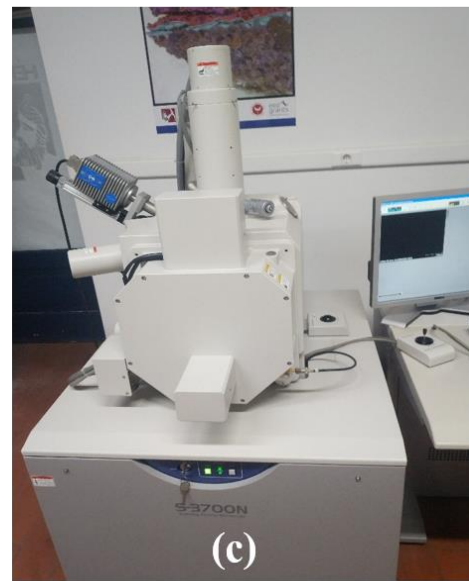
Fig. 3.8: SEM-EDX equipment utilized for surface characterization: (a) Servicio General de Apoyo a la Investigación, University of Zaragoza (Spain), (b) Laboratorio de Microscopías Avanzadas, University of Zaragoza (Spain), and (c) HERCULES Laboratory, University of Évora (Portugal).
