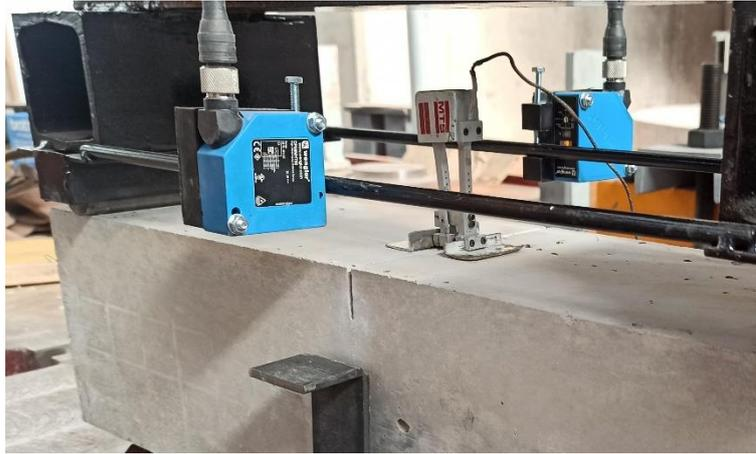
**Figure 3.2-15. Laser distance meters and axial extensometer placed on a specimen of size L.**
