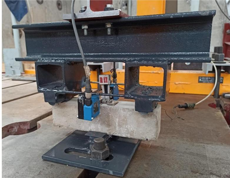
**Figure 3.2-14. Fixture for size S specimens.**
