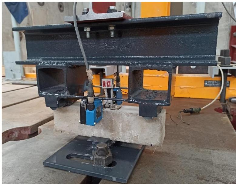
**Figure 3.2-4. Flexural strength test on a specimen of size S.**
