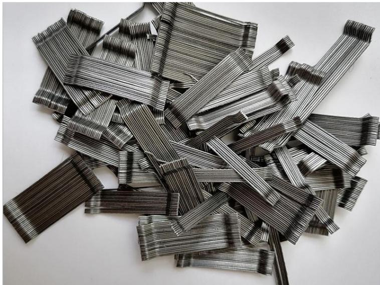
**Figure 2.1-1. Glued steel fibers with shaped ends.**
