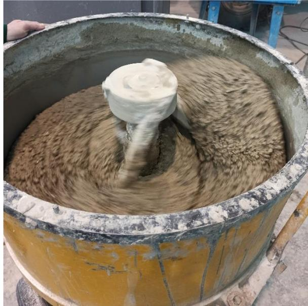
**Figure 3.1-8. Appearance of concrete with fibers at the end of the mixing time.**
