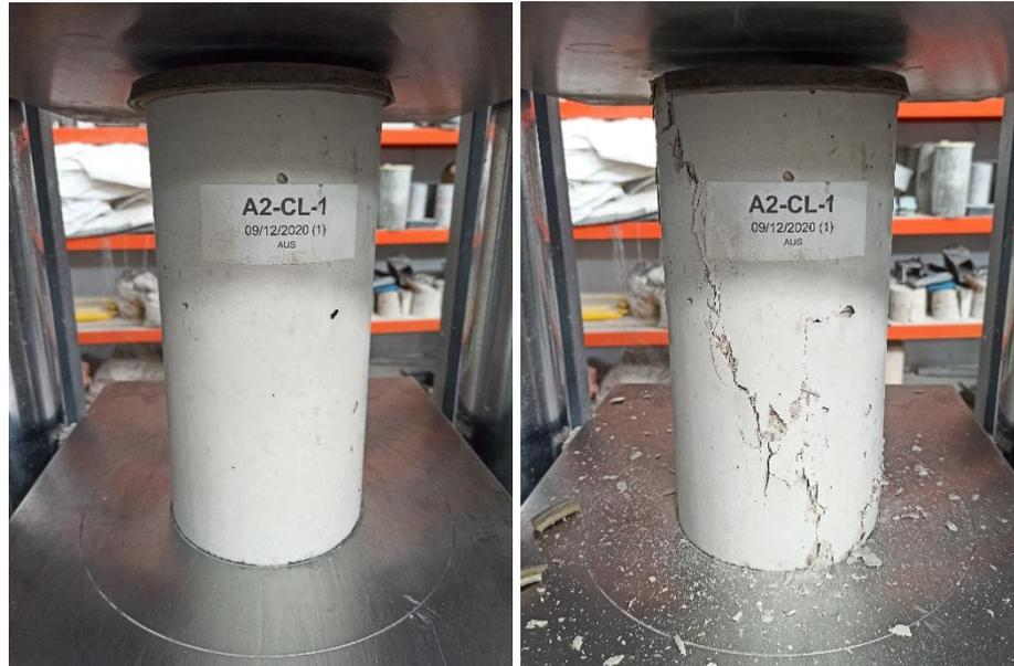
**Figure 3.2-2. Compressive strength test on a fiber-reinforced concrete specimen.**
