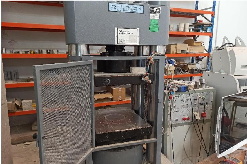
**Figure 3.2-11. 300 T testing machine.**
