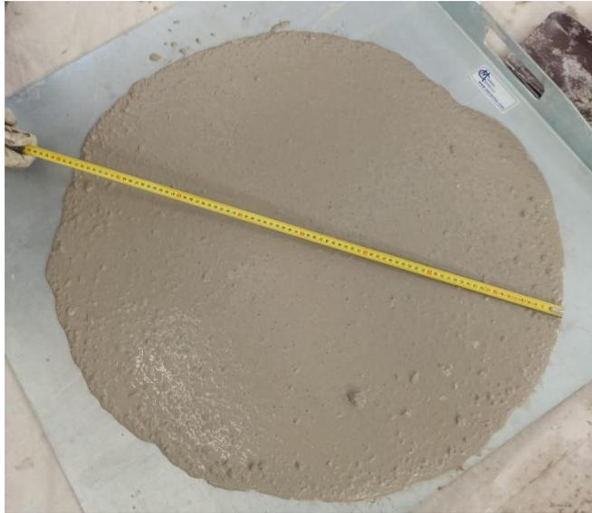
**Figure 3.2-1. Example of a slump test.**
