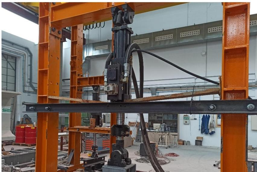
**Figure 3.2-12. 50 kN actuator positioned in its reaction frame.**
