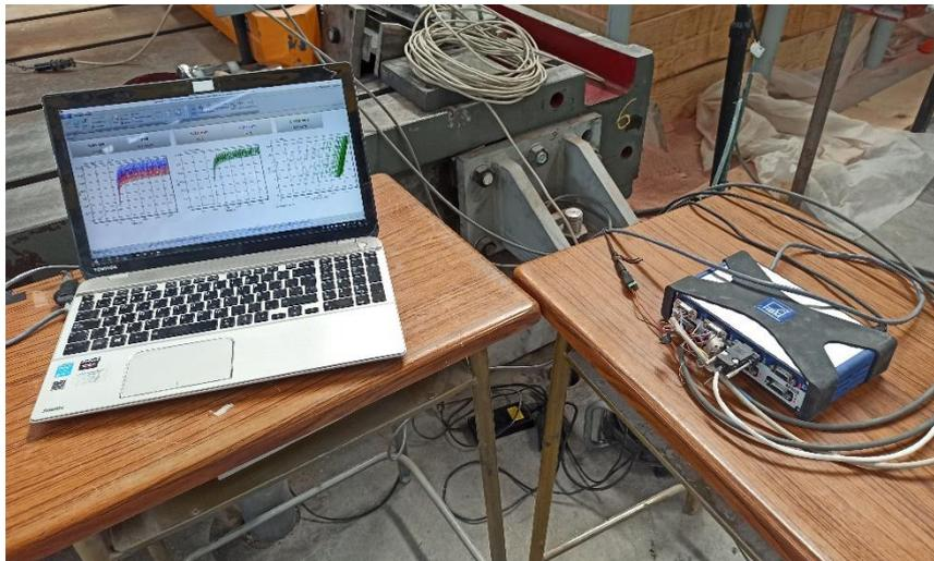
**Figure 3.2-16. Data acquisition with QuantumX module and Catman software.**
