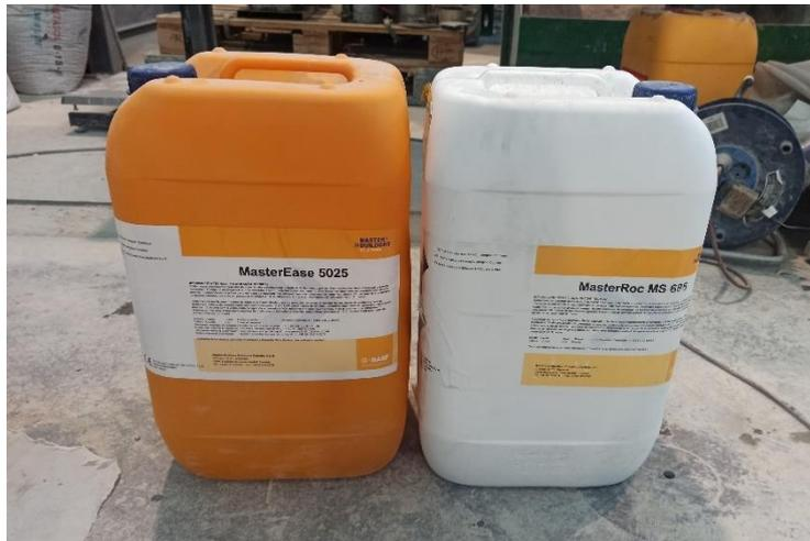
**Figure 3.1-1. Superplasticizer admixture (left) and nanosilica suspension (right).**
