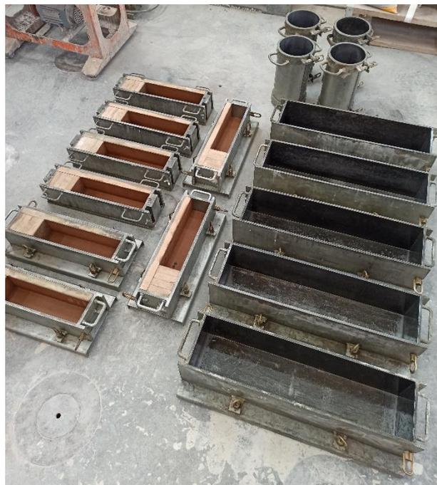
**Figure 3.1-5. Types of molds used: cylindrical 150x300 mm, prismatic 150x150x600 mm and prismatic 100x100x400 mm with reductions.**
