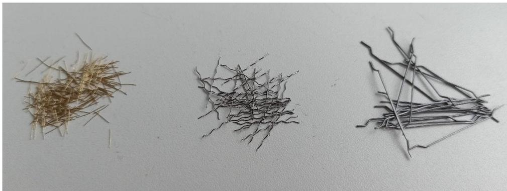
**Figure 2.1-3. Some of the most common types of steel fibers. From left to right, straight, crimped and hooked ends.**
