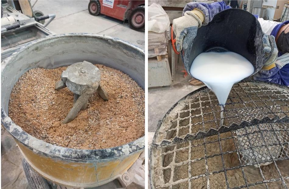
**Figure 3.1-7. Mixing of solid materials and addition of water with admixtures.**
