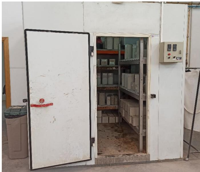
**Figure 3.1-9. Curing chamber used.**
