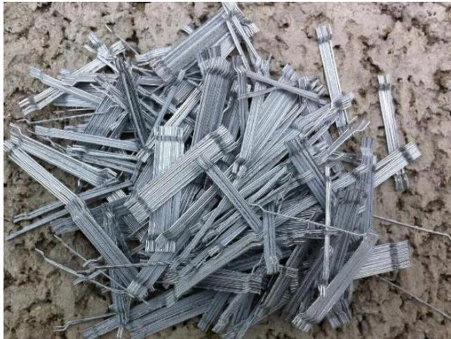
**Figure 3.1-2. Dramix RC-80/30-CP steel fibers.**
