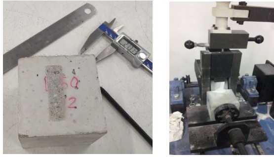
510 511 Figure 19. Abrasion test. Left: footprint on the M50 mix. Right: sample set up in the testing machine 512 In this research, the increase in fine RCA generated a cement paste with a lower surface hardness, 513 which increased the footprint size, as shown in Figure 20. These results were in line with the results of 514 the 90-day rebound index: a higher rebound index was produced in those mixtures with a smaller 515 footprint width (mix M75 had a lower rebound index, 39, and a footprint size of 21 mm that was 27.3 % 516 larger than the M0 footprint). Once again, there were two different groups of concretes, according to 517 the results of this test: high and low/medium fine RCA content.
