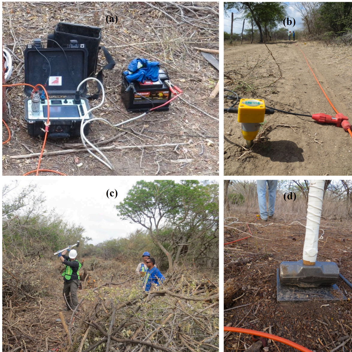
Fig. 1. Photos during some of the seismic refraction tests: (a) Seismographic acquisition equipment; (b) Geophone; (c) Depiction of the seismic excitation by a sledgehammer impact; (d) Sledgehammer with installed shock detector.
