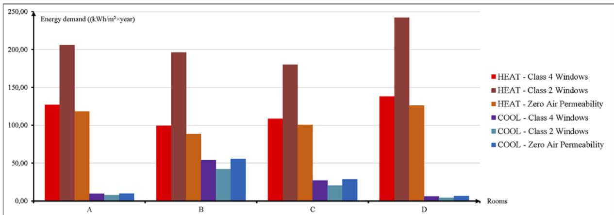
*Fig. 6. Results of the energy simulations related with the windows air permeability.*
