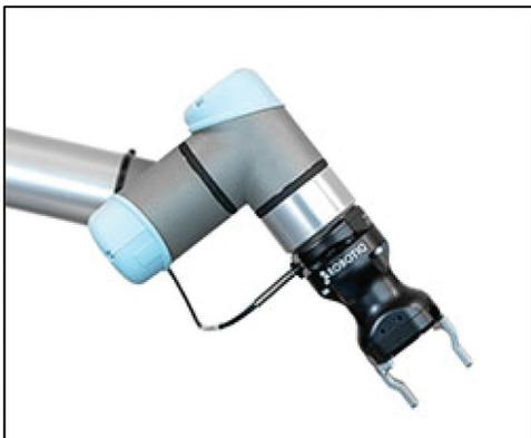
Figure 3. Cobot electric gripper.
