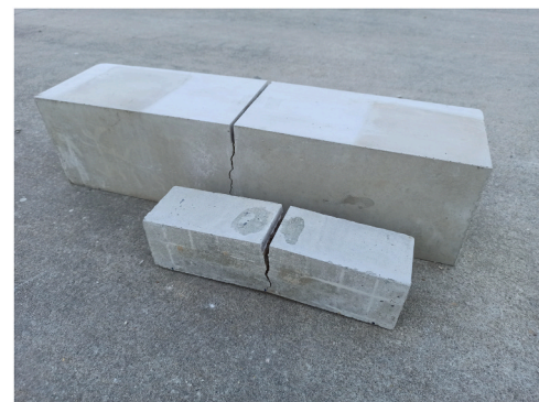
Fig. 2. Examples of real specimens of size S and L already tested.
