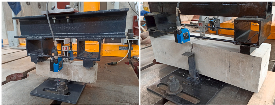
Fig. 3. Flexural test on specimens of size S (left) and L (right).
