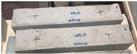
Fig. 7. Prismatic specimens for shrinkage test.
