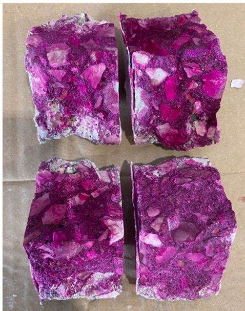
Fig. 5. Carbonation test samples.
