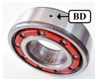
Figure 1.9: Induced Bearing Defect (BD) fault for the experimentation.
