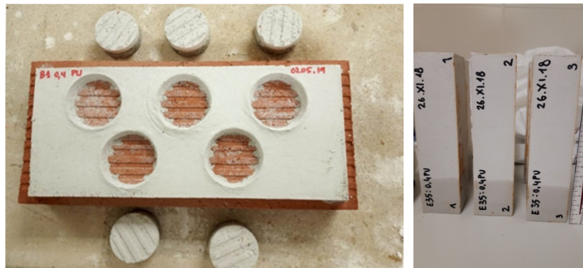
Figure 6. Adherence test (left), height of water after 10 min of the suction test (right)
