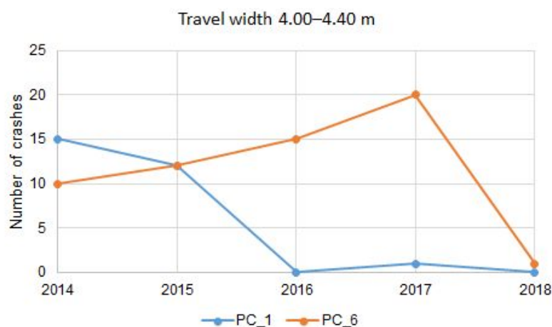
Figure 9. Trends in changes in number of crashes at pedestrian crossings in relation to the travel lane width.
