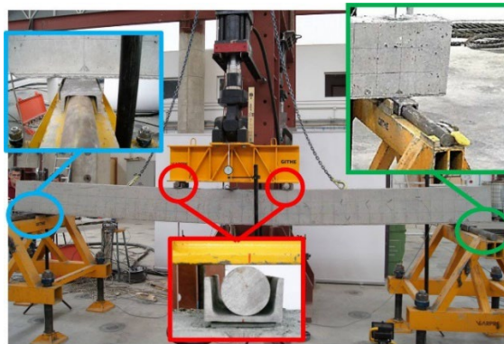
Figure 2: Four-point bending test image.
