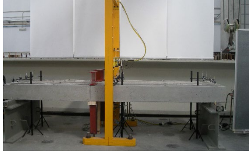
Figure 5: Arrangement of the beams in the long-term deformation test
