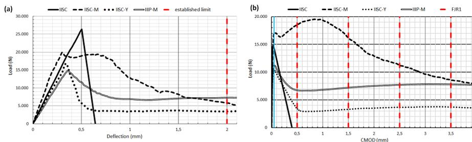
**Fig. 6.** Load versus deflection curves in: (a) four-point test; (b) three-point test
