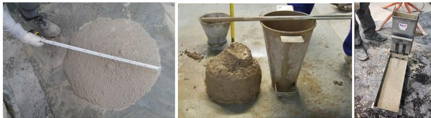
**Fig. 3.** From left to right: slump flow test, Abrams cone test and L-box test
