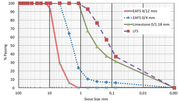
**Fig. 2.** Grading: aggregates and LFS
