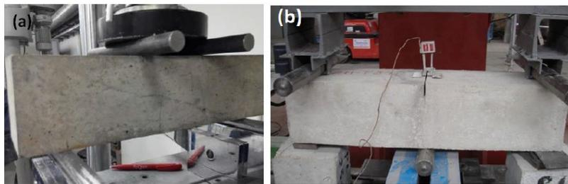
**Fig. 5.** Bending test set-up: (a) No notching four-point test; (b) Notching three-point test
