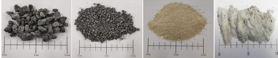
**Fig. 1.** Used aggregates and LFS: EAFS 4/12 mm (left); EAFS 0/4 mm (middle-left); limestone fines 0/1.18 mm (middle-right); LFS 0/1 mm (right).
