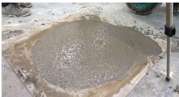
Fig. 1. Self-compacting concrete manufactured with EAF slag concrete
