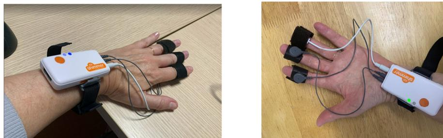
**Figure 2.** Example of the Shimmer3 GSR+ device.
