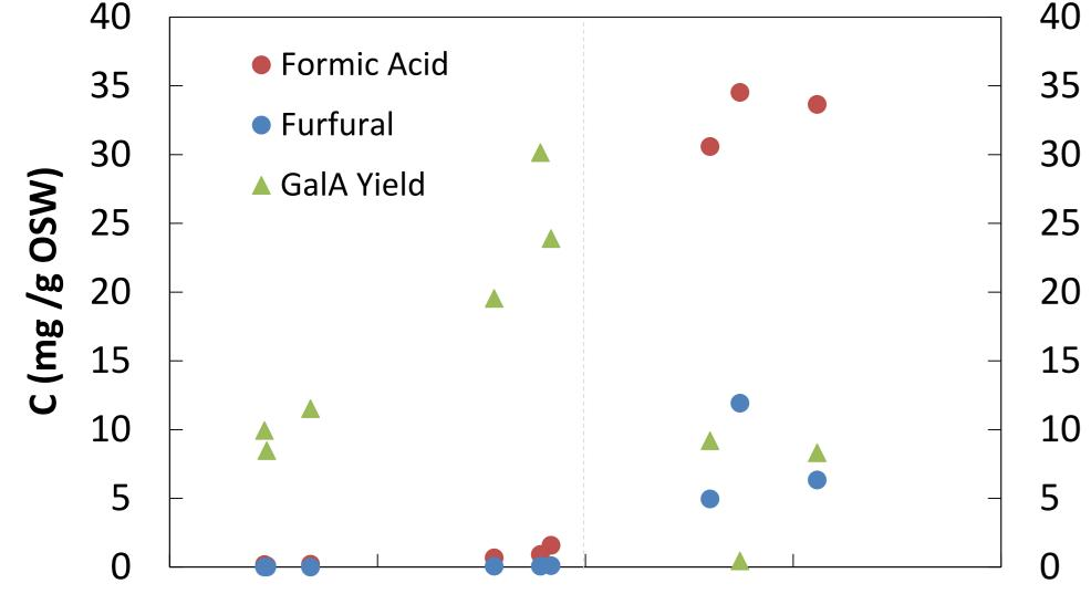
In the continuous reactor, a severity of 100 sets the boundary conditions: beyond this point, the yield drops, and degradation products are rapidly formed.
