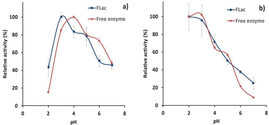
Fig. 5. Effect of pH on the free and immobilized laccase (FLac) from *M. thermophila* (a) and *T. versicolor* (b). Data are the arithmetic mean  $\pm$  standard deviation of three independent replicates.
