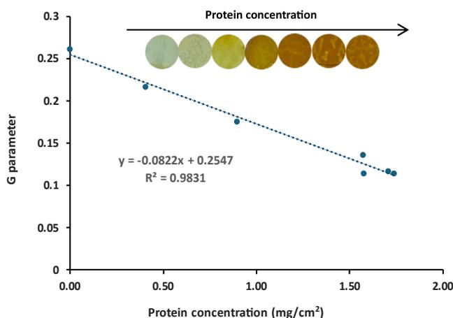
**Fig. 4.** Graphical representation of the G parameter from the photographed discs of laccase-polymer hybrid (*M. thermophila* laccase) versus protein concentration. At the top of the figure are the real images (photographs) of the discs, visually showing the color differences depending on the amount of protein anchored to the polymer.
