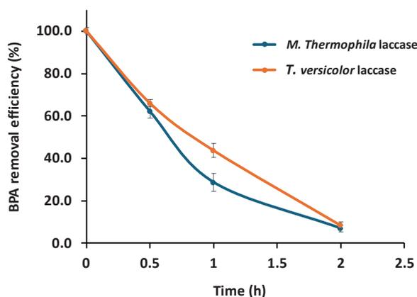
**Fig. 8.** Removal of BPA ( $80 \text{ mg L}^{-1}$  BPA in deionized water,  $25 \text{ }^\circ\text{C}$ ) by laccase-polymer hybrid (FLac) versus time. Error bars are related to standard deviation of triplicate test.
