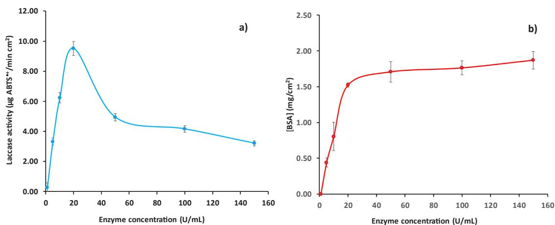
Fig. 3. Effect of the enzyme concentration on the laccase activity (a) and protein content (b) in the laccase-polymer hybrid (FLac). Immobilization time 1 h at 25 °C. U, units of commercial laccase from *M. thermophila*. Data are the arithmetic mean  $\pm$  standard deviation of three independent replicates.
