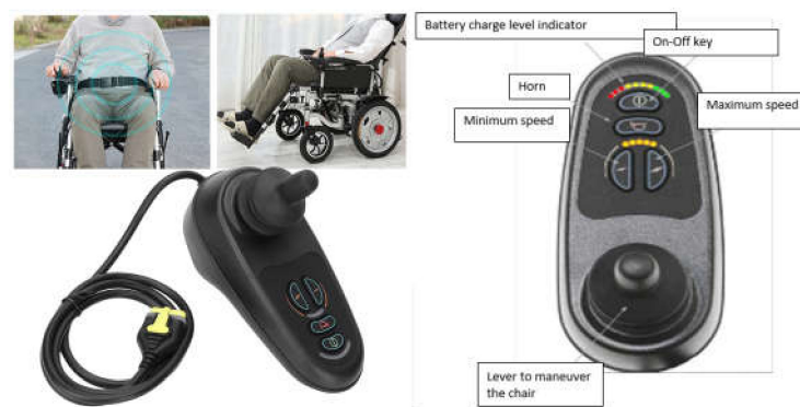
Figure 12. Manual control of motorized wheelchair.
