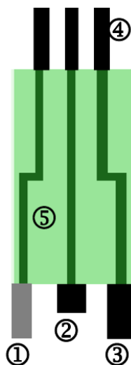
Figure 5.1. Diagram of the screen printed electrochemical system used. 1. Reference electrode; 2. Working carbon electrode; 3. Counter electrode; 4. Electrical connections; 5. Dielectric insulating layer.
