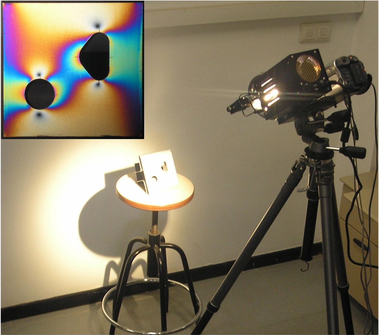
Fig. 3 Photograph of the experimental setup (the isochromatic fringe pattern observed through the polariscope is shown in the upper-left corner)
