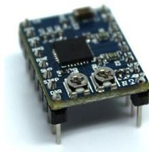
**Figura 60.** Driver de control de motor Paso a Paso - A4988 G3D Stepper Driver
